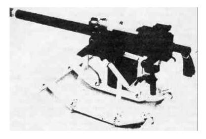
Figure 4-11 Machine-gun Mounted on a Toboggan
