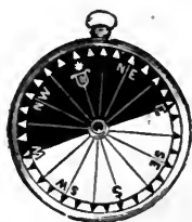
FIG. 46.—Barker's luminous compass.
