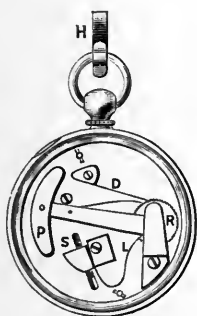
FIG. 300.—Construction of pedometer.
