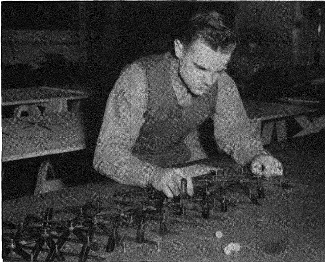
FIG. 176.—Laying up a strip of mechanical-triangulator assemblies.
