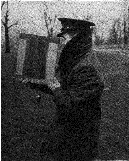
FIG. 45.—Determining slope by means of Abrams sketch board and a plumb bob.
