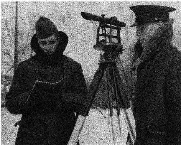
FIG. 24.—Reading and recording the doubled angle.
