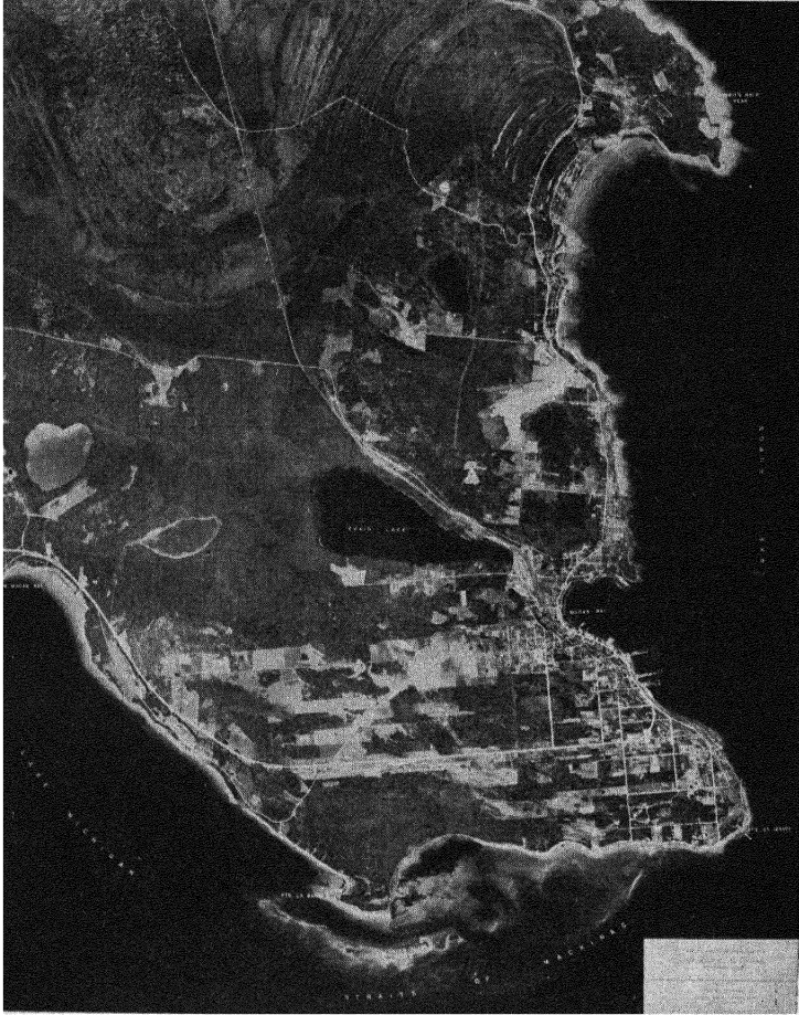
FIG. 181.—A semicontrolled mosaic laid to known horizontal distances.
