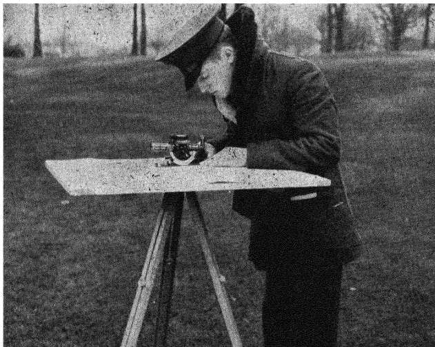
FIG. 39.—Using a plane table and alidade in the field for establishing control and topographic sketching.
