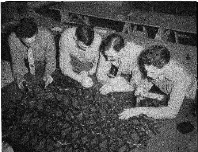
FIG. 177.—A complete mechanical-triangulator assembly lay-down.
