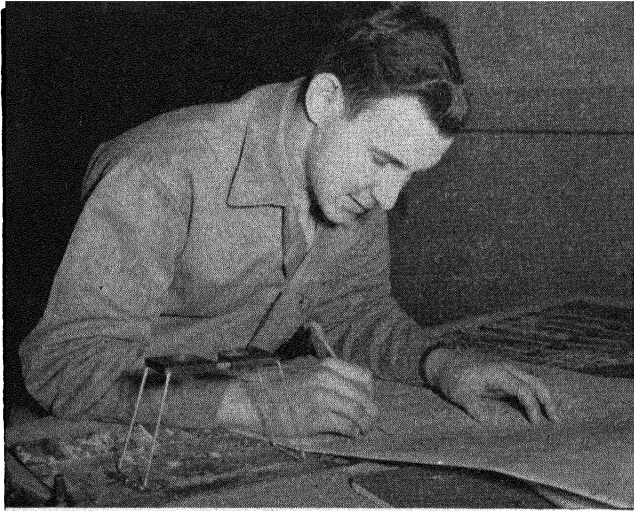
FIG. 163.—Identifying field control from a map by using a stereoscope with the photographs.
