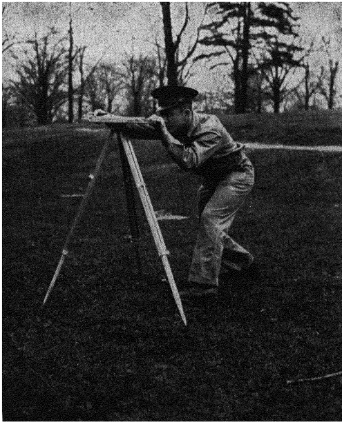
FIG. 44.—Student orienting the Abrams sketch board.
