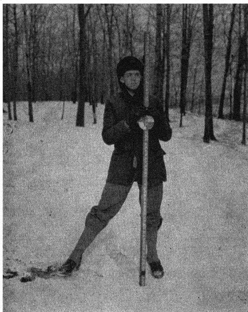
FIG. 37.—Student holding a level rod on a foresight to obtain vertical control.
