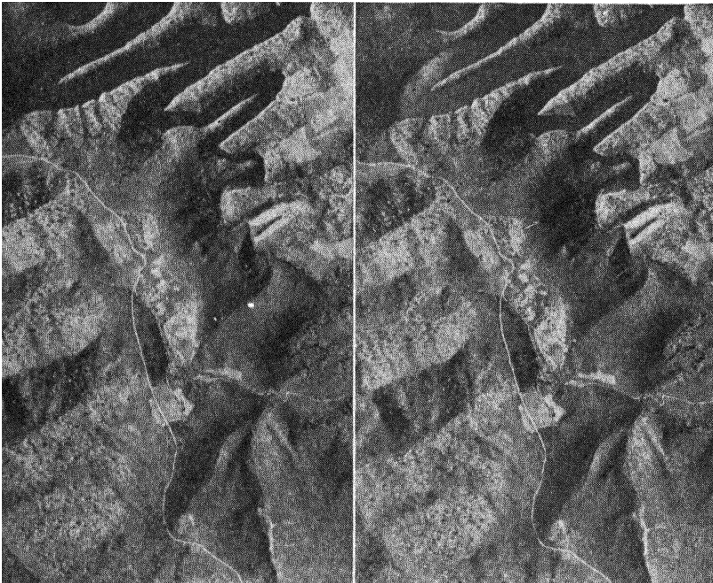
FIG. 101.—A stereogram properly oriented, spaced, and placed in position.
