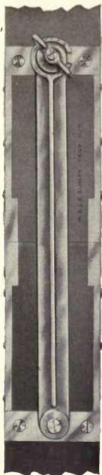
FIG. 70. VIEW OF HINGES, RIBBED BRACE AND CLAMP OF TELEMETER OR STADIA ROD
