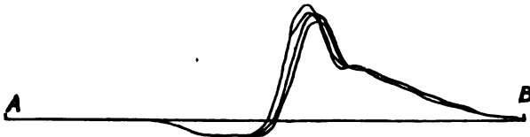
FIG. 236.—HUGON DIAGRAMS. Cylinder 8 inches, diameter 10 inch stroke. 75 rev. per minute. Scale 1 inch to 36 lbs.
