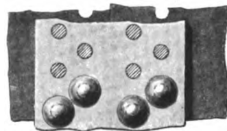
FIG. 155.—DOUBLE RIVETED BUTT-JOINT. TWO COVERING PLATES.
