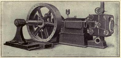
Fig. 44. Moderate Speed Engine of the Four-valve Type
