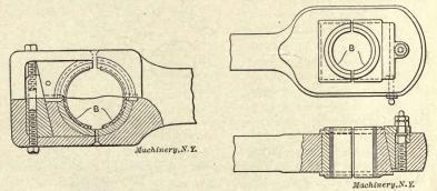
Figs. 32 and 33. Methods Commonly Used for Taking Up Wear in a Connecting-rod
