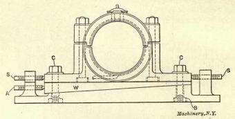
Fig. 34. Outboard Bearing for Corliss Type Engine
