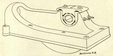
Fig. 35. Inner Bearing and Bed of Corliss Engine
