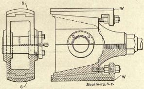
Fig. 31. A Typical Cross-head
