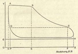
Fig. 53. Diagram for Calculating Steam Consumption
