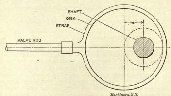
Fig. 10. Diagrammatical View of Eccentric
