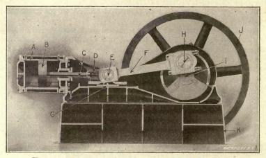
Fig. 1. Longitudinal Section through the Ames High-speed Engine
