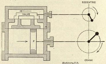
Fig. 15. Both Steam Ports Closed
