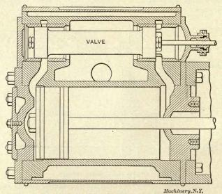
Fig. 17. Engine with Piston Valve
