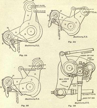
Figs. 23 to 26. Action of Corliss Valve Gear
