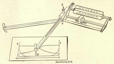
Fig. 52. General Construction of Planimeter
