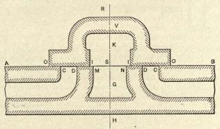
Fig. 8. Longitudinal Section of Slide Valve with Ports
