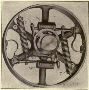
Fig. 37. Shaft Governor for High-speed Engine
