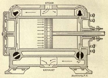
Fig. 20. Longitudinal Section through Corliss Engine
