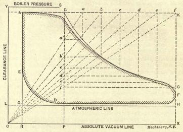
Fig. 7. Constructing a Steam Engine Work Diagram
