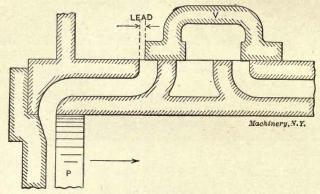
Fig. 9. Iliustration showing Lead of Slide Valve
