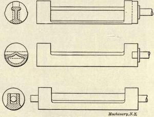
Fig. 19. Different Types of Corliss Valves
