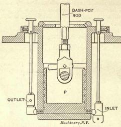
Fig. 28. Dash-pot for Corliss Engine
