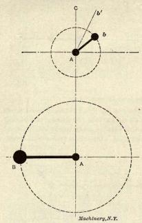
Fig. 11. Relations of Crank and Eccentric
