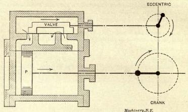
Fig. 12. Piston just beginning Forward Stroke
