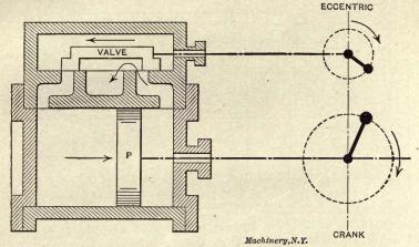
Fig. 14. Valve has started on Backward Stroke
