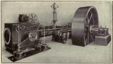
Fig. 45. The Harris Corliss Engine
