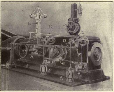
Fig. 22. The Monarch Engine with Corliss Valve Gear.—A, Rod to Eccentric; B, Governor; C, Reach Rod; D, Radial Arm; E, Steam Valve; P, Bell-crank; G, Wrist Plate; H, Exhaust Valve; K, Dash-pot
