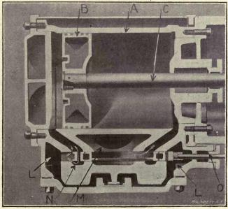
Fig. 2. Section of Cylinder, showing Slide Valve
