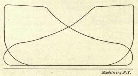
Fig. 50. A Typical Indicator Diagram
