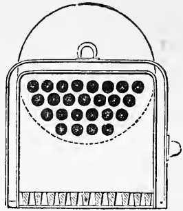
BOILER OF "ROCKET," 1829.
