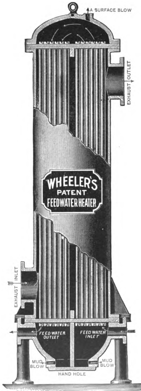
FIG 136.—Feed-water Heater.
