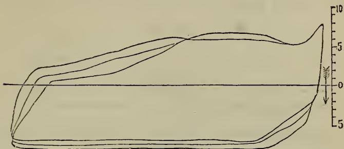
DIAGRAM FROM AIR-PUMP OF DUKE OF SUTHERLAND'S YACHT. (ORDINARY INJECTION.)
