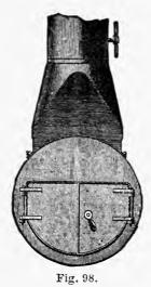
in combustion. They are made either of brick or metal; and usually have either an octagonal or circular cross-section. A circular, inside, cross-section is better than either a square or an octagonal cross-section, as it offers less resistance to the flow of the gases. A square, inside, cross-section is, really, equivalent only to a circular cross-section whose diameter is equal to that of a
