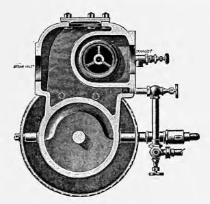
Fig. 16. Cross-section. Cylinder, Dick and Church Engine.
