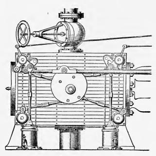
Fig. 20. Cylinder of Corliss Engine.
