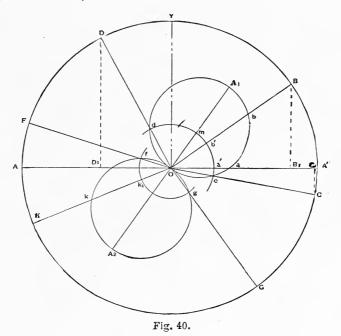
The value is open its maximum distance when the imaginary crank is in the position of the line  $OA_1$ , and then the value is at the right-hand end of its travel.
