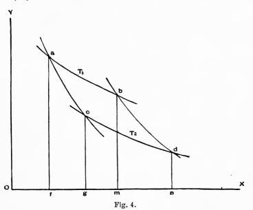
A comparison of the equation of the isothermal curve (15), with that of the adiabatic curve (24), makes it apparent that the latter is the steeper curve.
