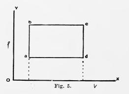
Suppose the working fluid is heated at the constant volume  $V_1$  until the pressure is  $P_2$ , and the absolute temperature is  $T_2$ . The line *ab* will represent the changes of volume and pressure during this process.
