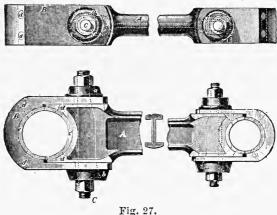
Fig. 27. Connecting Rod, Woodbury Engine.
