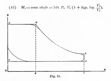
If we call  $P_{\rm m}$  the *mean forward pressure* in pounds per square inch on the piston during the forward stroke, then, since the work done is equal to the pressure per square foot multiplied by the volume swept through in cubic feet, we have
