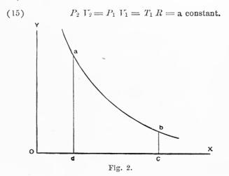
Equation (15) represents the law of the change of pressure and volume during isothermal expansion; and the curve represented by the equation, on the work diagram, is called the *Isothermal curve*, which for a perfect gas is the equilateral hyperbola.
