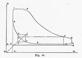
closed at 5. The part from 3 to 4 is made at the end of the stroke, when the pressure suddenly falls, from the final pressure of the steam after expansion, to almost the atmospheric pressure; and the part from 6 to I is made when the steam begins to enter the cylinder, just before the beginning of the forward stroke.
