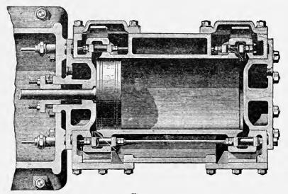
Fig. 18. Cylinder, Porter-Allen Engine.
