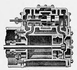
Fig. 15. Horizontal Section. Cylinder, Dick and Church Engine.
