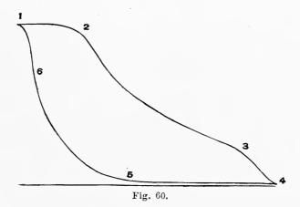
In the case of single valve engines, early admission and early exhaust may be corrected by turning the eccentric backward on the shaft, so as to reduce the angle of advance.
