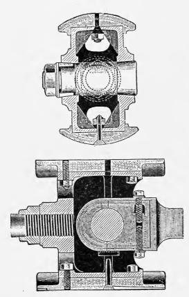
Fig. 23. Cross-head, Ide Engine.
