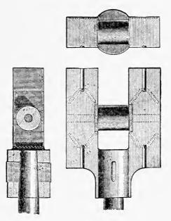
Fig. 22. Cross-head, Porter-Allen Engine.
