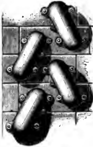
DISADVANTAGES OF PLACING RETURN BENDS OPPOSITE THE ENDS OF THE TUBES.
