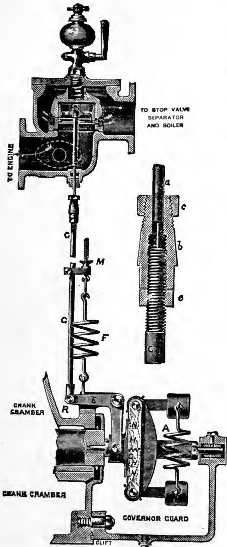
CENTRIFUGAL GOVERNOR FOR WILLANS' ENGINE.
