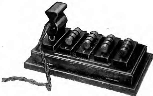
FIG. 3.—THERMOMETER SWITCHBOARD FOR ENABLING SEVERAL DIFFERENT TEMPERATURES TO BE TAKEN OR RECORDED.
