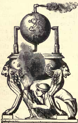
FIG. 1.—HERO'S ENGINE, B.C. 200.
