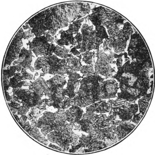
FIG. 13.—Peg quenched at 760° C. on cooling. x 100.
