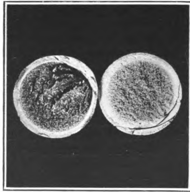
FIG. 20.—Fractures of bars quenched in water (right) and oil (left).
