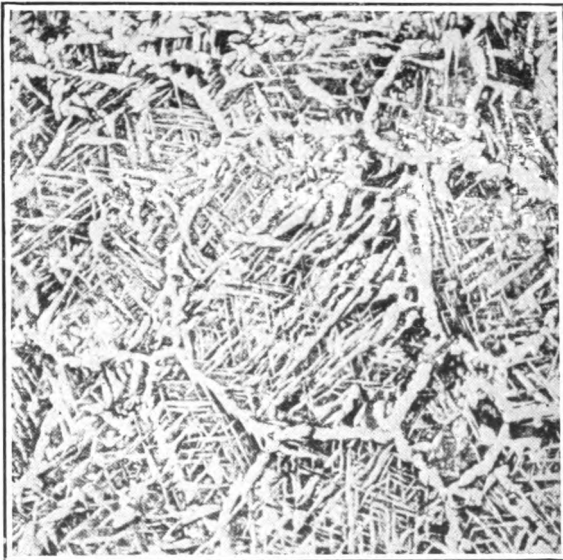
FIG. 3.—Overheated structure of mild steel. x 25.
