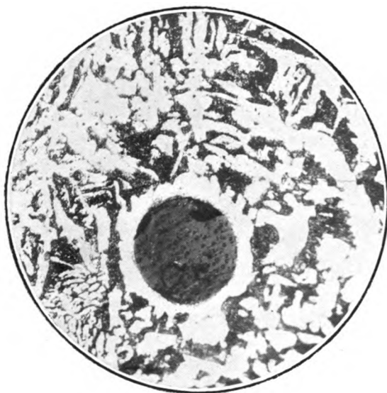
FIG. 25.— Slag globule in ferrite envelope. x 50.
