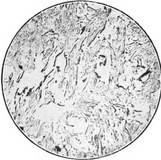
FIG. 45.—Thickening of carbide plates in pearlite areas due to slow cooling. x 200.
