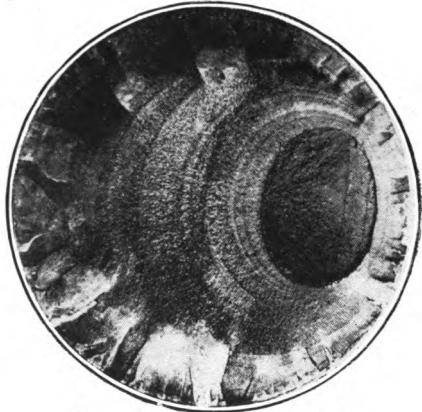
FIG. 68.—Creeping crack in waggon axle.
