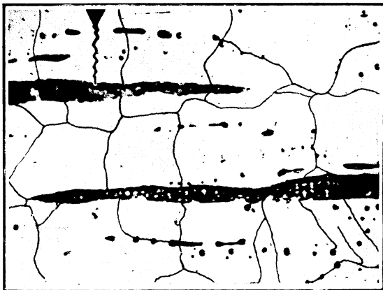
FIG. 23. --Wrought iron containing slag streaks. \times 150 .
