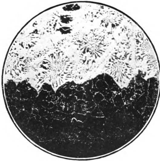
FIG. 61.—Microstructure of phosphide blister.
