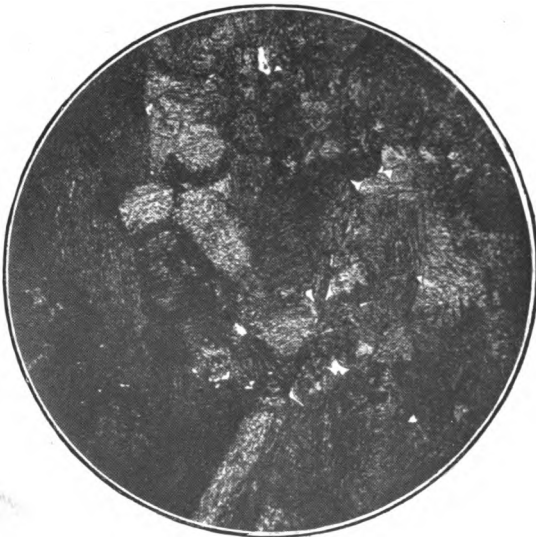
FIG. 12. —Peg quenched at 800^{\circ}\text{C} . on cooling. \times 100 .
