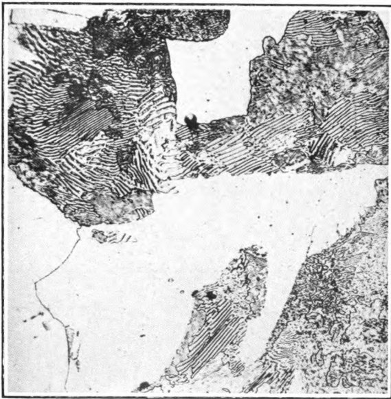
FIG. 15.—Peg quenched at 670^{\circ}\text{C} . on cooling. \times 800 .
