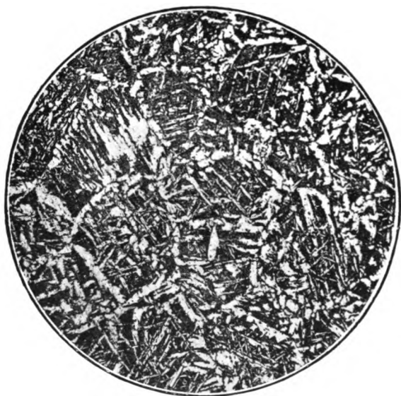
FIG. 8.—Peg quenched at 780° C. on heating. x 25.
