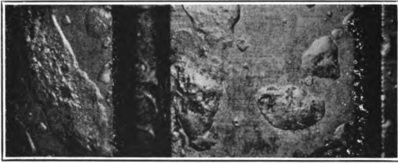
FIG. 60.—Phosphide blisters on cemented gear.
