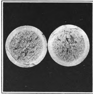
FIG. 19.—Fine crystalline core in case-hardened bar.
