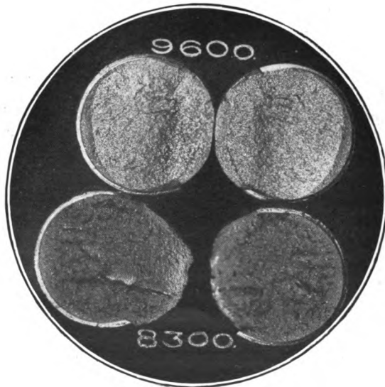
FIG. 69.—Forces needed to break bars having crystalline and “fibrous” cores.
