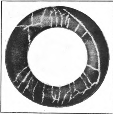
FIG. 40.—Cracks in flat surface of ground washer.
