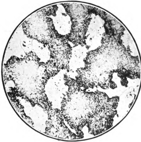
FIG. 35.—Troostite fringes within the core. x 200.
