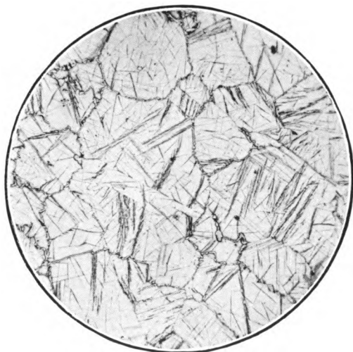
FIG. 30.—Cementite in needles and cell walls in quenched specimen. x 300.
