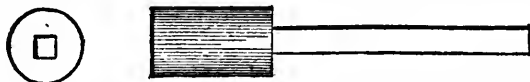
Making a Valve Yoke by the Method of "Novis Homo." Fig. 250—Side and End Views of the Stem after Drawing.
