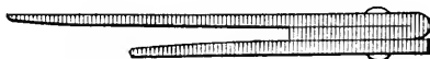
Fig. 349—Showing how the Two Pieces of Steel are Bolted Together Ready to Draw Out.
