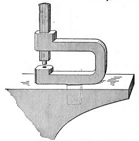
FIG. 71.—THE ANVIL PUNCH COMPLETED.
