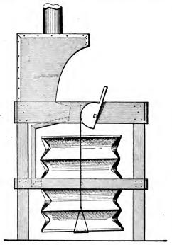
FIG. 48.—HOME-MADE PORTABLE FORGE.
