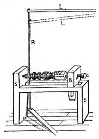
FIG. II-A PRIMITIVE LATHE.
