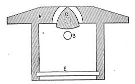
FIG. 50 IS A SECTIONAL VIEW THROUGH SLAG BREAKER D.
