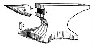
FIG. 54.--PUTTING A HORN ON AN ANVIL BY THE METHOD OF "C. H."
