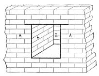
FIG. 26.—SHOWING HOW THE RECESS IS MADE.
