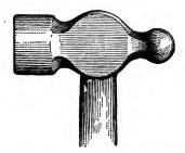
FIG. 85.--THE BALL PANE HAMMER.
