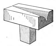
FIG. 169.—SHOWING A TOOL FOR MAKING HARROW TEETH.
