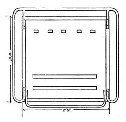
FIG. 34.-TOP VIEW OF WORK BENCH.
