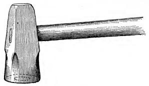
FIG. 117.—THE CUPPING TOOL.
