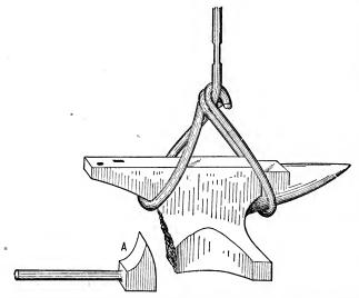
FIG. 59.—THE ANVIL AND THE PIECE USED IN MENDING IT.
