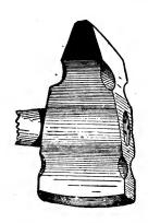
FIG. 4-THE LONG CROSS-FACE HAMMER.
