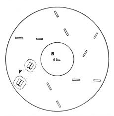
FIG. 201.—SIDE PLATES, BETWEEN WHICH FANS ARE FASTENED.
