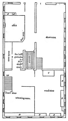
FIG. 52.--PLAN OF THE FIRST FLOOR. AA, Closets. BBB, Benches. C, Rack.
