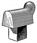
FIG. 124.—THE BOTTOM FULLER.
