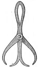
FIG. 86.—THE DOUBLE CALIPERS.
