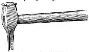
FIG. 113 .-- THE SQUARE CHISEL.
