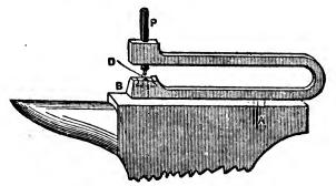
FIG. 67.—PUNCH MADE BY "H. S."
