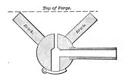
FIG. 196.—IMPROVED TUYERE, AS MADE BY "IRON JACK."
