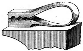
FIG. 66.—SELF-ACTING SWEDGE DESIGNED BY "E. M. B."
