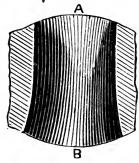
FIGS. 75 AND 76.—CORRECT SHAPE OF EYE FOR TOOL-HANDLE.
