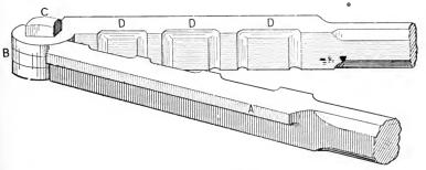
FIG. 189 .-- TOOL USED IN MAKING CLIPS.
