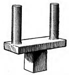
FIG. 130.—A FORK USED IN BENDING.
