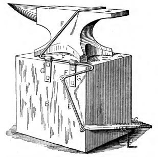
FIG. 58.—DEVICE FOR HOLDING WORK ON THE ANVIL.
