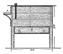
FIG. 42 .- SIDE VIEW OF BENCH, SHOWING DIMENSIONS.
