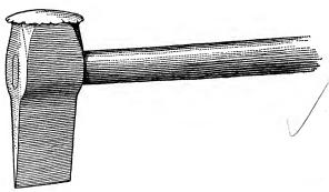
FIG. 109.—THE HOT CHISEL.
