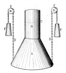
FIG. 16-THE SMOKE-STACK AND BONNET.
