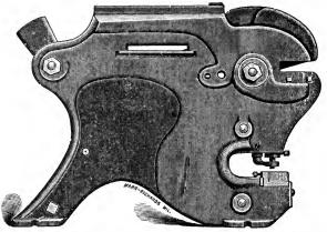
COMBINED PUNCH AND SHEAR, for heavy work. Cuts flat Bar ½ by 4, 5% by 3, ½ by 2, 1 inch round or less. Also cuts Plow Steel ½ by 6. Punches ½ inch thick—all without any change. Three sets of knives and one punch all independent of each other. Weight, 650 pounds. Punches to center of 8 inches. Price, \$85.00.
