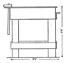
FIG. 35.-END VIEW OF WORK BENCH,
