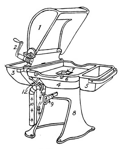
FIGURE 1. NAMES OF PARTS OF FORGE.
