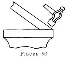
than the bottom. This gives the proper clearance. The point is bent upward to give the proper rake.
