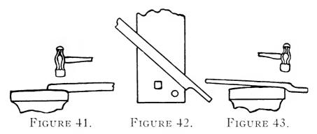
*Third*—Form second step. Turn the work to the left and form shoulder even with the first, on the sharp edge of the anvil. Hold at about 60° as shown in Figure 42.
