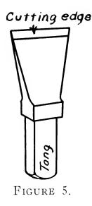
The Hardie. The Hardie is a tool used about the anvil for cutting hot and cold iron. (Figure 5.)
