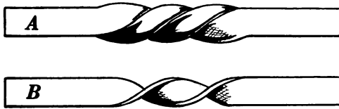
FIG. 41. — A, METAL TWISTED WHILE HOT; B, METAL TWISTED WHILE COLD.
