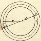
be measured along the center of the stock, as shown by the dotted line. It is the diameter of this circle, made by the dotted line, that is used for calculating the length of stock; and for convenience this may be called the "calculating" di-
