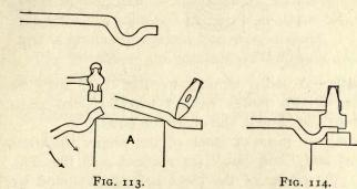
The eye may be flattened with the set-hammer, and the part between the jaw proper and the eye worked down to shape over the horn and on the anyl with the same tool.
