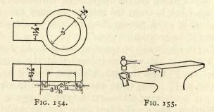
To make this, a flat bar is forged rounding on the end, punched and split as shown. The split is widened out by driving a punch, or other tapering tool into it, and the forging finished by working over the horn of the anvil, as shown in Fig. 155.
