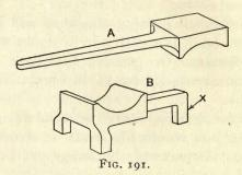
for an anvil-die having a square hole, similar to the hardie-hole in an ordinary anvil, near one end. The horn on the swage, at x, slips into this hole, while the other two projections fit, one on either side, over the sides of the anvil. These horns, or fingers, prevent the swage from slipping around when in use.
