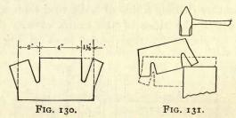
These ends are then forged out round in the manner illustrated in Fig. 131. The forging should be placed over the corner of the anvil in the position shown, the blows striking upon the corner of the piece as indicated. As the end gradually straightens out, the other end of the piece is slowly raised into the position shown by the dotted lines and the shaft hammered down round and finished up between swages.
