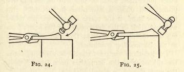
24. This drives the metal back and makes a sort of thick ridge at the beginning of the scarf. In finishing the scarf, use the flat face of the hammer, and bring the piece to the very edge of the anvil, as in this way a hard blow may be struck without danger of hitting the anvil instead of the work. The proper position is shown in Fig. 25.
