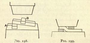
are two pieces of flat iron of the same thickness. The stock is placed like Fig. 198, the hammer brought down lightly, to make sure that everything is in the proper position, and then one hard blow bends the stock into shape (Fig. 199).
