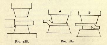
work should be so placed as to work in the shoulder with the top die, while the bottom die keeps the under side of the work straight, as in Fig. 189, A. The same object, a shoulder on one side only, may be accomplished by using a block, as shown at B, Fig. 189. The block may be used as shown, or the positions of work and block may be reversed and the work laid with flat side on the anvil and block placed on top.
