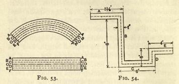
length of the line following the center of the stock of the bent shape.
