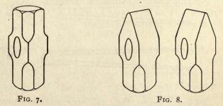
Sledges are also made with a cross-pene or straightpene, as shown in Fig. 8.
