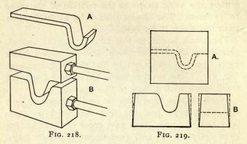
pine and then sawing to shape with a band-saw. The block was "laid off" as shown in Fig. 219, A, the sawing being done on the dotted lines. This left the blocks of such a shape that the space between them, when they were brought together with the upper and lower edges parallel, was just equal to the thickness of the stock to be bent.
