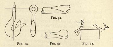
The next step is to round up the part for the eye, as shown in Fig. 92, by forming it over the corner of the anvil as indicated in Fig. 93. The eye should be forged as nearly round as possible, and then punched.
