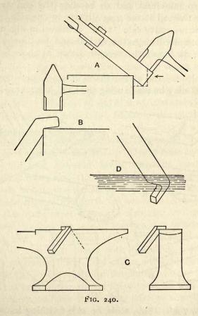
This end is further bent by holding and striking as illustrated at B. The diamond shape is given to the end by swinging the tool back and forth and striking as shown at C, which gives a side and end view of tool in position on the anvil.
