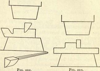
very deep, they should first be made with a hotchisel and then spread with the spreading tool. If the shoulder is not very high, both operations, of cutting and spreading, may be done at once with the spreading tool.
