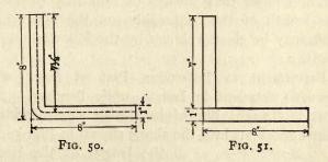
Suppose this to be made of wood in place of iron. It is easily seen that a piece of stock  $\mathbf{I}''$  thick and  $\mathbf{I5}''$  long would make the angle by cutting off 7''
