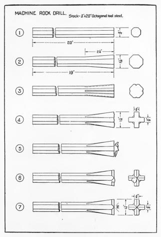
a square set-hammer. Trim off the end of the drill with a very thin hot chisel, making it square, as shown at 5.
