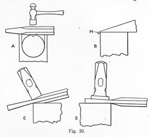
Harden and temper the cutting edge in the same manner as the flat chisel.
