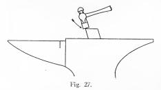
Cutting Cold Stock.—In cutting cold bars of soft steel or wrought iron with a cold chisel the method employed should be as follows: Around the bar make a series of cuts about one-fourth of the way thru, taking care to have them always at right angles to the axis of the bar. Tilt the bar slightly, and place the partly cut section at the outer edge of the anvil. By hitting the projecting end a sharp blow with a sledge it should break off easily.
