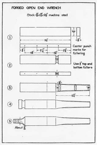
the jaws of the tongs from being caught between the dies. It is therefore best to use a piece of stock  $9\frac{1}{2}$  inches long. This will give enough material for two wrenches, with an allowance for a short tong hold. Remember to use hollow-bit tongs. Flat-jawed tongs are unsafe.
