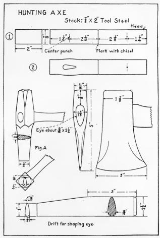
side, the punch should be removed and cooled. Punching is then finished from the other side.
