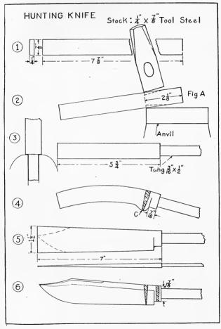
**ĤARDENING.**—The knife is heated slowly in a piece of pipe in the same manner as the tap. When it has reached the refining heat it is dipped in fish oil, the back or thick edge first, and cooled quickly.
