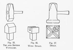
V-fullers shown in Fig 55. The stock should be turned during this operation, to insure uniformity in the depth of the fuller cuts.
