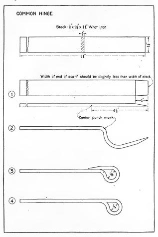
STEP FOUR.—In placing the piece in the fire have the scarf down, in order to avoid burning the eye. When the piece is at the welding heat, it should be removed from the fire and laid on the anvil with the scarf up and the eye against the rounded edge of the anvil. If this were not done and it were welded over the sharp edge of the anvil, the neck would have a sharp corner instead of being rounded, as shown at 4. The welding is done with a heavy hand-hammer.
