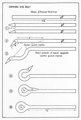
slightly larger than the finished hole, in the eye and bring the scarf and shank together, as at 5.
