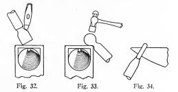
with a 1/2-inch top-swage. Make the hole circular by driving a tapered pin thru it. The finished eye should then appear as if made from round stock.
