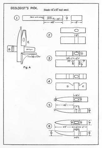
manner. It is tempered to a brown or a dark straw color. In heating the head, care should be taken to prevent the heat from flowing back and softening the hardened point. This may be done by keeping damp coals around the point.
