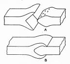
Fig. 42. Split Weld for Heavy Stock,
