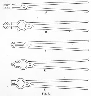
A, flat-jawed; B, hollow-bits; C, link; D, pick-ups; E, chisel.
