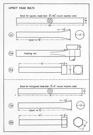
hot end on the face of the anvil, holding the piece vertically with a pair of link-tongs, and strike on the cold end with a heavy hand-hammer. Care should be taken to keep the stock straight while upsetting.
