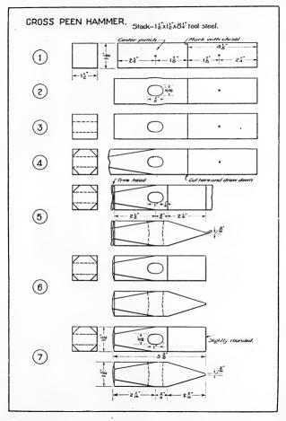
was done with the cold chisel. When it has cooled enough, the peen is hardened in the same manner, care being taken not to cool the stock around the eye. While cooling the peen, water should be allowed to drip on the center of the face. This prevents the colors from running down before the peen has been cooled enough, and insures a uniformly hardened face. If the face were cooled by merely dipping it in water, the outside edges would harden faster than the center and be more likely to crack.
