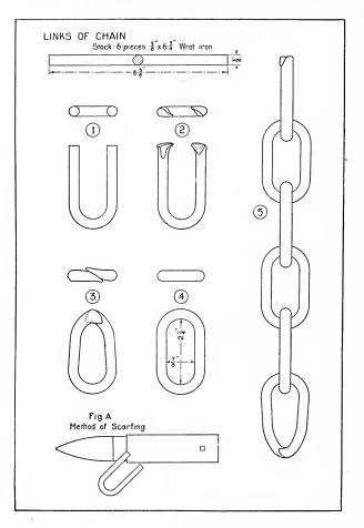
it points to the left, the scarf is left-hand and is harder to weld. The link should be shaped so that the end to be welded is narrower than the other. The stock is then less liable to be hammered small on either side of the weld, and the semicircular end will be about the right size when the weld is finished.
