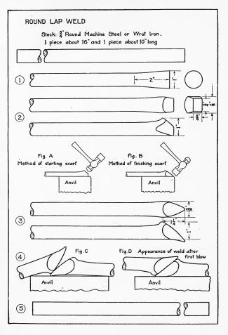
piece. The end of one scarf should lap over the thick ridge, or heel, of the other, as in Fig. D.
