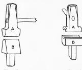
Fig. 18 Fig. 19. Top and Bottom Fuller. Top and Bottom Swage.
