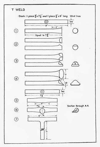
smoothed between top- and bottom-swages, and the scale removed with a file. The ends are then trimmed off, making the dimensions of the T as shown at 7.
