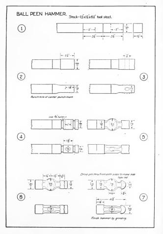
sides, in order to insure a square end. Draw-out the face, swage it, and trim it with a hot chisel. The peen should then be cut to length, and the corners cut off. It is rounded in a bottom-swage. The reason for finishing the face before the peen is that it is hard to hold the peen with a pair of tongs.
