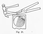
end, A, of the link is then heated, the scarfs spread apart, as shown in Fig. 31, the links slipped on, and the scarfs brought together again. This connecting link is welded in the same manner as the others.
