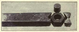
Fig. 37. Showing how a Hexagon Nut is produced from Rectangular Bar in a Hot-pressed Nut Machine
