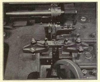
Fig. 23. View looking down into Die Space of Ajax Continuousmotion Bolt and Rivet Headen
