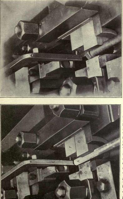
Fig. 6. First Step in the Production of Bolt Heads in Plain Forging Dies of the Type shown in Fig. 3
