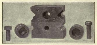
Fig. 12. Combination Square and Hexagon Double-deck Bolt Dies
