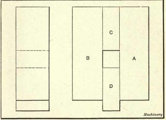
Fig. 43. Type of Dies used in making Square Nuts in Machine of the Type shown in Fig. 32
