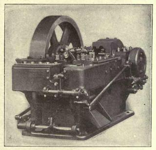
Fig. 14. Two-inch National Wedge-grip Bolt and Rivet Header
