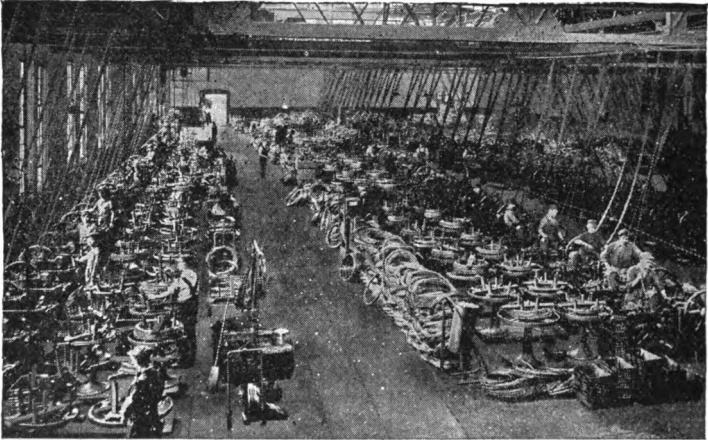
FIG. 109.—A Nail Factory. The wire is fed into machines which cut and shape the wire into nails.
