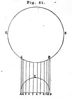
Let the circle OH, fig. 51, equal the large pipe, AB, CD, the Branch or Collar; describe the semicircle AEB; divide the semicircle into any number of equal parts; from the points, draw lines parallel to AC, as 1, 2, 3, &c.
