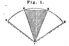
Let ABI be the given cone. From I as centre, with the radius IA, describe the arc CD; make CD; equal in length to the circumference of AB (which can be found by a reference to the table of the *Circumferences of Circles*;) draw the lines CI and DI; then the figure CDI will be that of the required surface of the cone.
