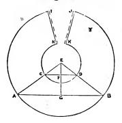
Let AB equal diameter of can, or base of a flange; CD diameter of opening in the top; FG altitude. Produce AC and BD until they meet at E; with E as centre, and the radii ED and EB, describe the curves IJ and HK; set off IJ equal to the circumference of the base AB; draw the lines IH and JK, cutting the centre at E.
