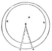
Describe a circle one inch larger in diameter than the hoop after the edge is laid off; lay the hoop on the plate, allowing an edge each side, as shown by the distance between the two circles and the dot on the line AC, the circle DE representing the hoop; take the distance from A to the dot on the line AC, and set off three times the distance on the outer circle, as from A to B'; draw the lines AC and BC, cutting the centre at C.
