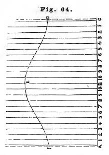
Set off the line ABC, fig. 64, equal in length to the circumference of the Elbow AB; erect the perpendicular lines AF, BE and CD; set off on each side of BE the same number of equal distances, as in the semicircle AGB; from the points draw lines parallel to BE, as 1, 1, 2, 2, 3, 3, &c.; make BE equal to BF; make AF and CD equal to AE; also, each of the parallel lines bearing the same figures as 1, 1, 2, 2, 3, 3, &c.
