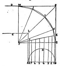
Let ABED, fig. 69, be the given elbow; draw the line FC; make FL equal in length to one-half the diameter of the elbow, with F as a centre; describe the arc GM; divide the arc GM into four equal parts, and draw the lines FJ and FH; also, the line IH; divide the section GH into two equal parts, and draw the line FK; draw the line AB at right angle to BC; describe the semicircle ANB; divide the semicircle into any number of equal parts; from the points draw lines parallel to BC, as 1, 2, 3, &c.
