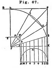
Let ABED, fig. 67, be the given elbow; draw the line FC; make FM equal in length to one-half the diameter of the elbow, with F as a centre; describe the arc KL; divide the arc KL into three equal parts; draw the lines FH and FI; also the line IH divide the section HK into two equal parts, and draw the line FG; draw the line AB at right angles to BC; describe the semicircle ANB; divide the semicircle into any number of equal parts, from the points draw lines parallel to BC, as 1, 2, 3, &c.
