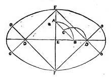
On the intersection of the two diameters as a centre, with a radius equal to one-half the difference of the two diameters, describe the arc AB, and from B as a centre, with half the chord ACB, describe the arc CD; from E as a centre with the distance ED cut the diameters at FF and DD; draw the lines FO, FO, FO, FO; then from F and F as centres, describe the arcs OO, and OO; also, from D and D as centres, describe the smaller arcs, OO and OO, which will complete the ellipse as required.
