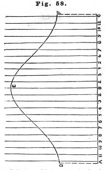
Then set off the line ABC, fig. 58, equal in length to the circumference of the cylinder CE; erect the perpendicular lines AD, BE and CF; set off on each side of BE the same number of equal distances, as in the semicircle CDE; from the points draw lines parallel to BE; make BE equal to BE; make AD and CF equal to FC; also, each of the parallel lines bearing the same number as 22, 33, 44, &c.; then a line traced through the points will form the pattern.
