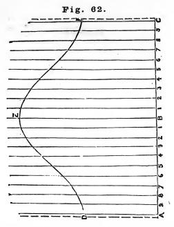
Set off the line ABC, fig. 62, equal in length to the eircumference of the elbow AB; erect the perpendicular lines AD, BE and CF; set off on each side of BE the same number of equal distances, as in the semicircle AGB; from the points draw lines parallel to BE; make BE equal to BC; make AD and CF equal to AF; also, each of the parallel lines bearing the same figures as 11, 22, 38, &c.; then a line traced through the points will form the pattern.
