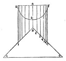
Let ABC, fig. 59, equal the pitch of a roof; let DF, IH, be the pipe; draw the line BG parallel to HF; draw the line DF at right angle to HF; describe the semicircle DEF; divide one-half the semicircle into any number of equal parts; from the points draw lines parallel to FH, as 2, 3, 4, &c.
