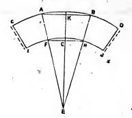
Let AB equal diameter of large end; FH diameter of small end; GK altitude. Produce AF and BH until they meet at E; with E as centre, and the radii EF and EA, describe the arcs CD and IJ; set off CD equal to that portion of the circumference of AB required for a pattern; draw the lines CI and DJ, cutting the centre at E.
