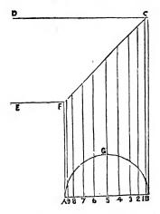
Let ABCD, fig. 61, be the given elbow; draw the line AB at right angles to BC; draw the line FC; describe the semicircle AGB; divide the semicircle into any number of equal parts; from the points draw lines parallel to BC, as 1, 2, 3, &c.
