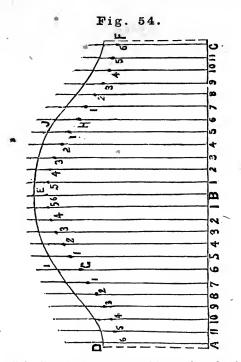
Set off the line ABC, fig. 54, equal in length to the circumference of the collar, CE; erect the lines AD, BE and CF; set off on each side of BE the same number of equal distances, as in the semicircle, and from the points draw lines parallel to BE, as 11, 22, &c.; make BE equal to AC in fig. 53; make AD and CF equal to BE; also, each of the parallel lines bearing the same figures; make GI and HJ equal to CF; also, each of the parallel lines bearing the same figures as 11, 11, 22, 22, &c.
