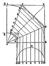
Let ABED, fig. 65, be the given elbow; draw the line FC; make FK equal to one-half the diameter of the elbow, with F as a centro; describe the arcs GL; divide the arc GL into four equal parts; draw the lines FH and FJ; also, the line JH; draw the line AB at right angles to BC; describe the semicircle AMB; divide the semicircle into any number of equal parts; from the points draw lines parallel to BH, as 1, 2, 3, &c.
