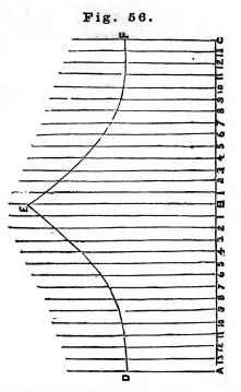
Set off the line ABC, fig. 56, equal in length to the circumference of the collar AB; erect the perpendicular lines AD, BE and CH; set off on each side of BE the same number of equal distances, as in the semicircle ACB; from the points draw lines parallel to BE; make BE equal to EB; make AD and CF equal to DA; also, each of the parallel lines bearing the same figures as 11, 22, 33, &c.; then a line traced through the points will form the pattern.
