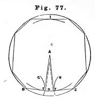
Describe a circle, three-quarters of an inch larger in diameter than a circle that will cut each corner of the article the top or cover is for; set off the squares from B to C; take one half of the largest square; and with B and C as centres, describe arcs G and H; then with A as centre, describe the arc cutting the square at I and the arc D; where the arcs GD and HD intersect, draw the lines AE and AF, also the lines BE and CF.
