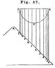
Let AB, fig. 57, equal the angle of the roof of a building; let CE, FB equal the pipe; draw the line CE; describe the semicircle CDE; divide the semicircle into any number of equal parts; from the points draw lines parallel to EB, as 2, 3, 4, &c.
