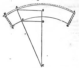
Describe the right angle ABE; make BD the altitude; draw the line CD at right angle to BE; make AB equal one-half the diameter of the large end, CD one-half the diameter of the small end; draw a line cutting the points A and C, and the line BE with E as a centre and the radius EC and EA describe the arcs FG and HI; set off FG equal to that portion of the circumference of the smallest end required for a pattern; draw the lines HF and IG, cutting the centre at E.
