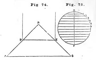
Let ABC, fig. 74, be the pitch of the roof; make DE equal to the diameter of the pipe; describe the circle FG; make FG the same in diameter as the pipe; draw the line FG; set off on the line FG any number of equal parts; from the points draw lines at right angle to FG as 1, 2, &c.
