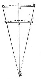
Multiply the slant height by one-half the diameter of the large end, and divide the product by one-half the difference of the two ends, and the quotent is the radius; the versed sine is found by multiplying the altitude by one-half the diameter of the large end; and dividing the product by one-half the difference of the two ends; then substract the quotent from the radius, and the remainder is the versed sine.
