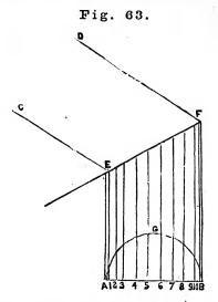
Let ABCD, fig. 63, be the given Elbow; draw the line AB at right angle to BF; draw the line EF; describe the semicircle AGB; divide the semicircle AGB into any number of equal parts; from the points draw lines parallel to BF, as 1, 2, 3, &c.
