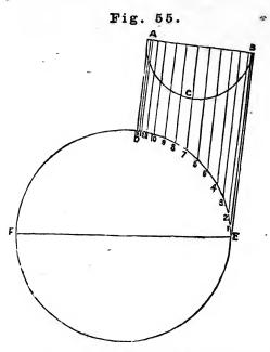
Let the circle FE, fig. 55, equal large pipe or boiler; make AB equal to the diameter of the collar or branch pipe, BE the angle required; describe the semicircle ACB; divide the semioircle into any number of equal parts; from the points draw lines parallel to BE, as 1, 2, 3, &c.
