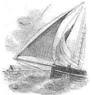
top of the lower mast. The JIB AND PORD HAIL OF A BLOOP. Only sail that rises above the lower mast is the gaff. In stormy weather this sail is always taken down. If the wind increases to a gale, the jib is lowered and lashed to the bowsprit.
