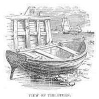
The keel may be formed by running melted lead into a groove cut in a piece of wood, or, better still, into a groove made in nearly dry clay. By driving four or five nails (well greased) into the groove before pouring in the melted lead, holes may be formed in the keel by simply withdrawing the nails after it is cold.
