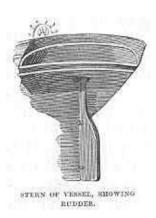
The *stern-post* rises from the opposite end of the keel, and also slopes a little outwards. To it are fastened the ends of the planking and the framework of the
