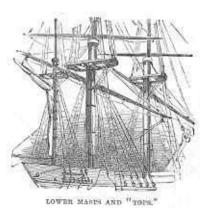
The parts of the different masts are connected and secured by means of *cross-trees* and *caps*, which are named after the mast and part of the mast to which they belong. Thus we have the *fore-top*, the *fore-top-mast cross-trees*, the *main-top*, and *main-top-mast cross-trees*, etcetera. Observe, particularly, that the *fore-top*, *main-top*, and *mizzen-top*, are the platforms, or cross-trees, at the tops of the *lower-masts*, and not—as might well be supposed by landsmen—the extreme tops
