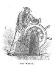
The *wheel*, which has been already referred to, stands usually at the stern of the ship, on the quarter-deck; but it is sometimes placed on an elevated platform amid-ships, so that the steersman may see more clearly where he is going.
