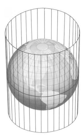
Figure 304. A cylindrical projection.
