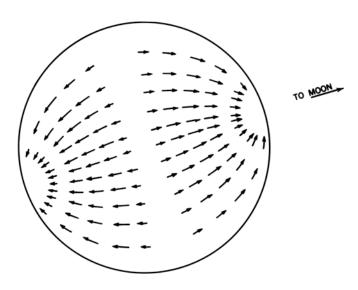
Figure 903b. Tractive forces across the surface of the Earth.
