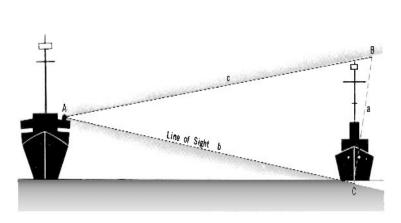
Figure 811c. Principle of stadimeter operation.
