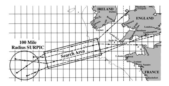
Figure 2814. Example of the use of a radius SURPIC to locate ships to search a rectangular area.
