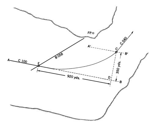
Figure 802b. Allowing for advance and transfer.
