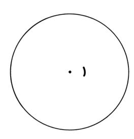
Figure 1307e. Position of second-trace echo on 12-mile range scale after changing PRR.
