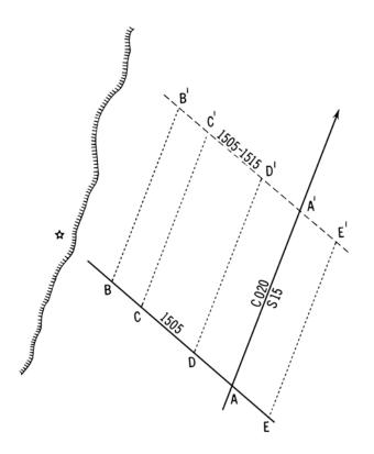
Figure 812a. Advancing a line of position.
