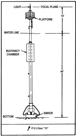
Figure 501b. Typical design for a buoyant beacon.
