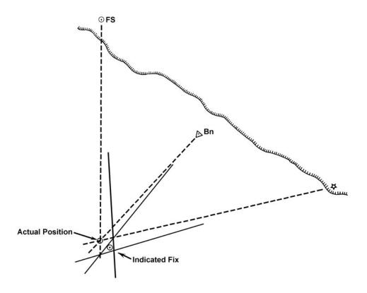
Figure 824. Adjusting a fix for constant error.
