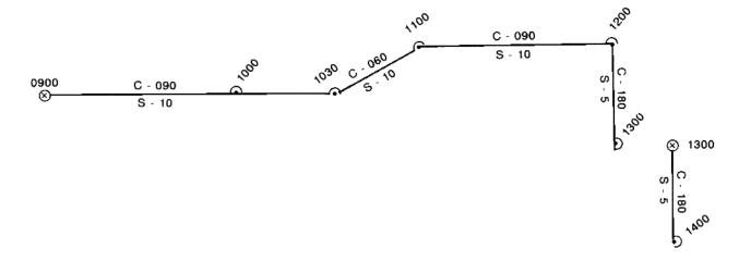
Figure 703. A typical dead reckoning plot.
