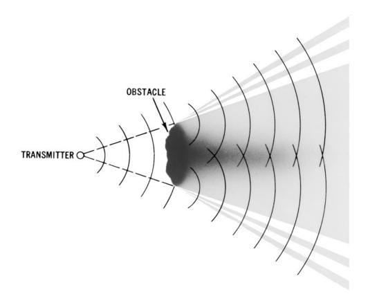
Figure 1008. Diffraction.
