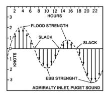
Figure 914b. Reversing tidal current.
