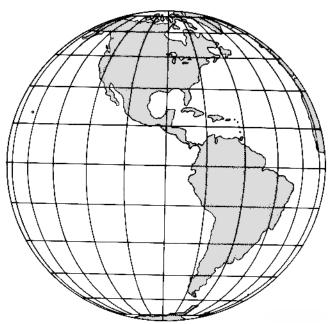
Figure 318a. An equatorial orthographic projection.
