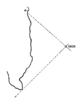
Figure 811a. A fix by two bearing lines.
