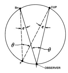
Figure 823a. Two-bearing plot.
