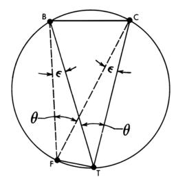
Figure 823b. Two-bearing plot with constant error.
