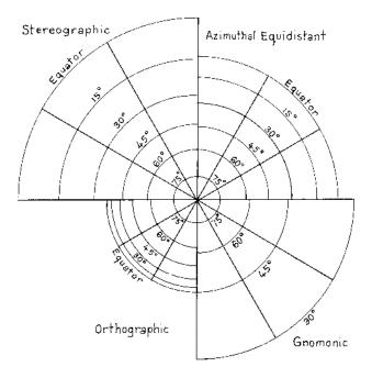
Figure 320. Expansion of polar azimuthal projections.
