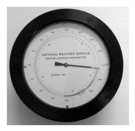
Figure 3602. An aneroid barometer.
