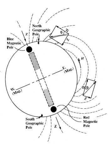
Figure 602a. Terrestrial magnetism.
