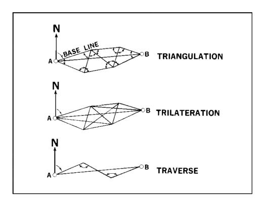
Figure 206. Triangulation, trilateration, and traverse.
