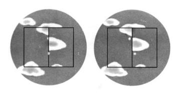
Figure 1612b. Testing the perpendicularity of the horizon glass. On the left, side error does not exist. At the right, side error does exist.
