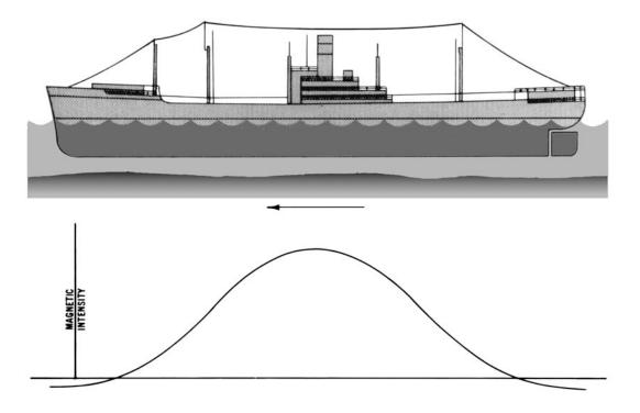
Figure 611b. A simplified signature of a vessel of Figure 611a.
