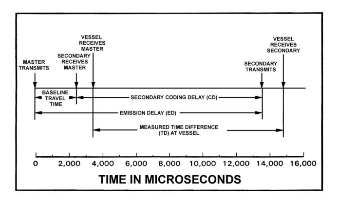
Figure 1203b. The time axis for Loran TD for point "A."
