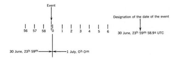
Figure 1817b. Dating of event in the vicinity of a negative leap second.
