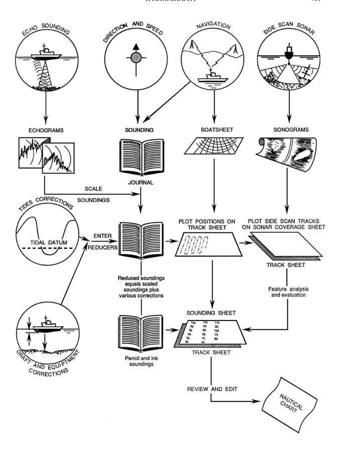
Figure 2904. The process of hydrographic surveying.
