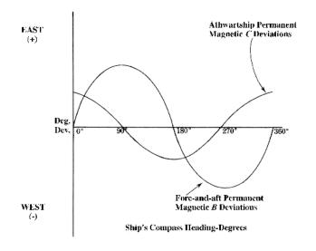
Figure 604b. Permanent magnetic deviation effects.
