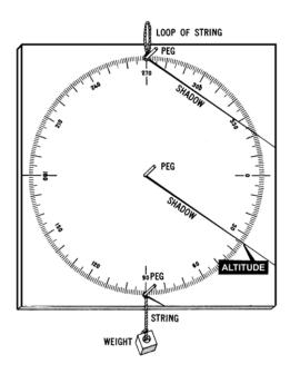
Figure 2608a. Improvised astrolabe; shadow method.
