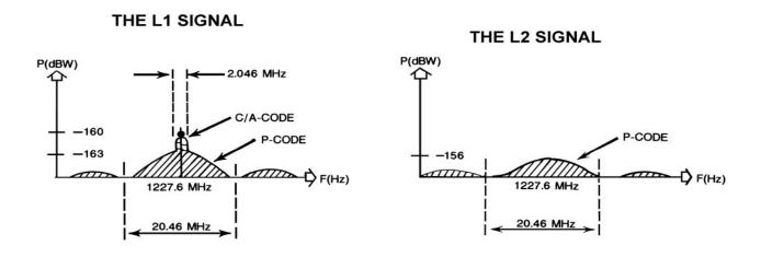
Figure 1104b. Modulation of the L1 and L2 carrier frequencies with the C/A and P code signals.
