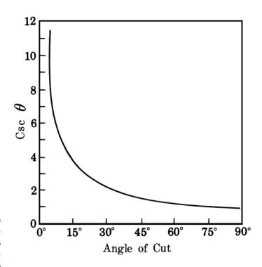
Figure 823c. Error of two-bearing plot.
