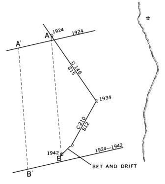
Figure 812b. Advancing a line of position with a change in course and speed, allowing for set and drift.
