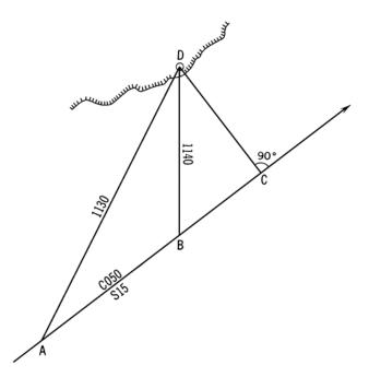
Figure 821. Triangles involved in a Table 18 running fix.
