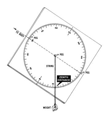
Figure 2608b. Improvised astrolabe; direct sighting method.
