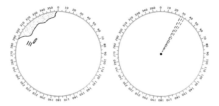
Figure 1308b. Coded racon signal.
