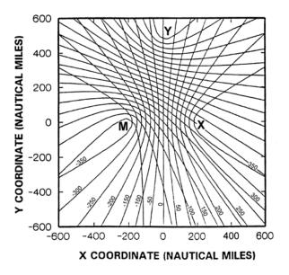
Figure 1208b. A hyperbolic lattice formed by station pairs M-X and M-Y.
