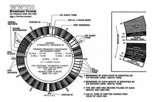
Figure 1816b. Broadcast format of station WWVH.
