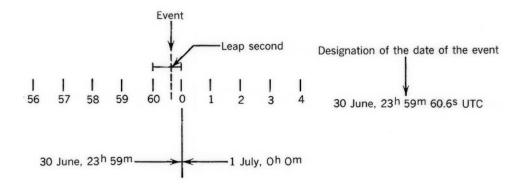
Figure 1817a. Dating of event in the vicinity of a positive leap second.
