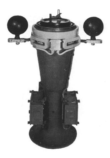
Figure 616. Type K degaussing compensation installation.
