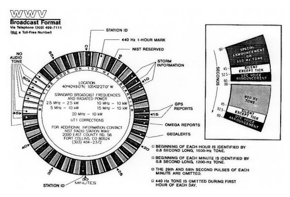
Figure 1816a. Broadcast format of station WWV.
