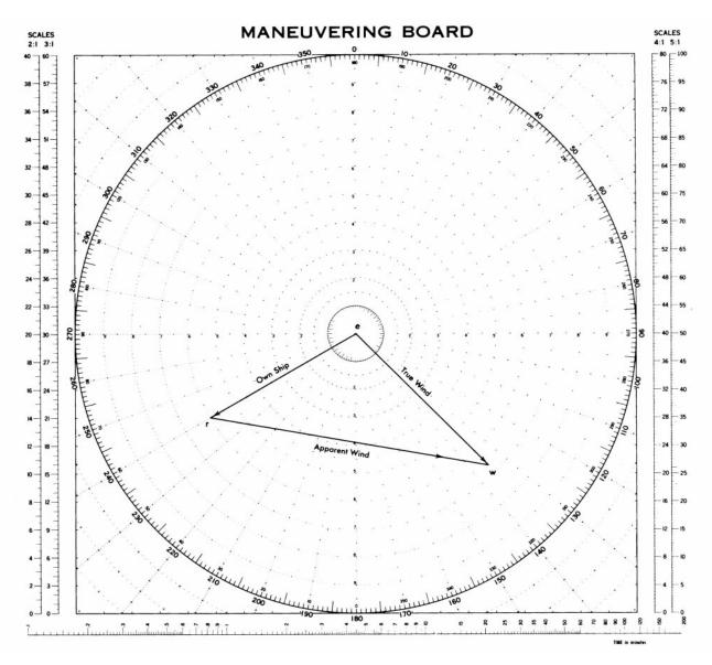
Figure 3609. Finding true wind by Maneuvering Board.
