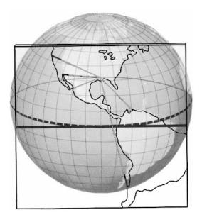
Figure 317a. An equatorial stereographic projection.
