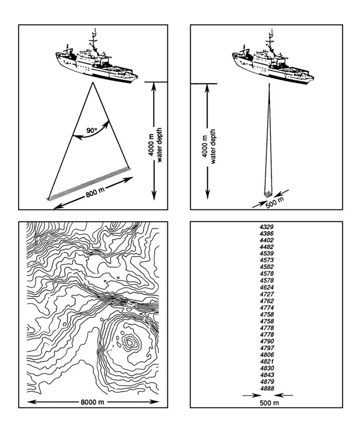
Figure 2905. Swath versus single-transducer surveys.
