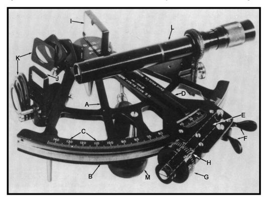
Figure 1602. U.S. Navy Mark 2 micrometer drum sextant.
