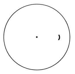
Figure 1307d. Second-trace echo on 12-mile range scale. Figure 1307e. Position of second-trace echo on 12-mile
