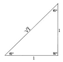
Figure 2108c. Numerical relationship of sides of 30°, 60°, and 45° triangles.
