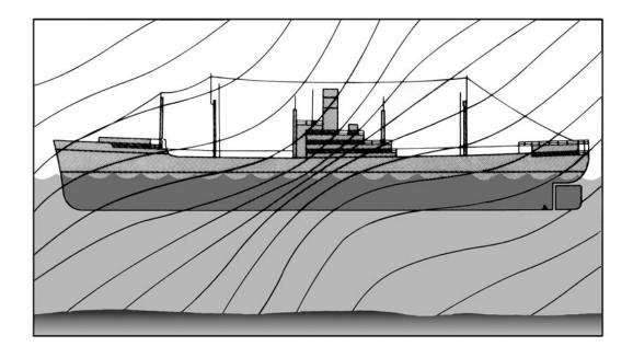
Figure 611a. Simplified diagram of distortion of Earth's magnetic field in the vicinity of a steel vessel.
