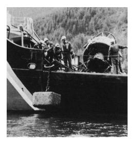
Figure 512. A sinker used to anchor a buoy.
