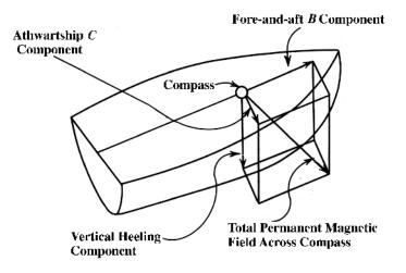
Figure 604a. Components of permanent magnetic field.
