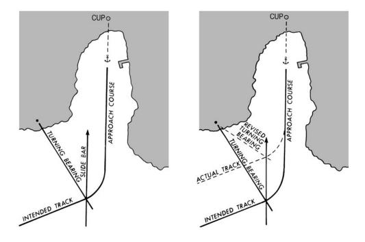
Figure 802c. The slide bar technique.
