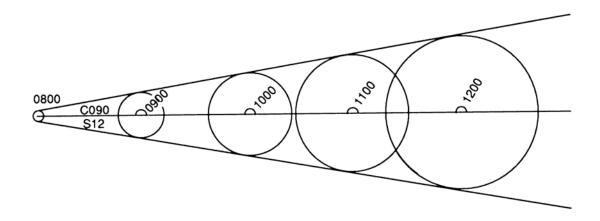
Figure 705. Fix expansion. All possible positions of the ship lie between the lines tangent to the expanding circles.
