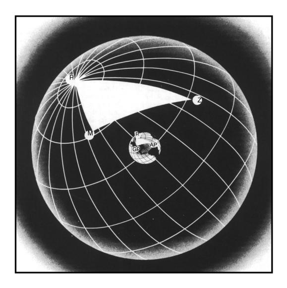
Figure 1529b. The navigational triangle in perspective.
