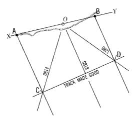
Figure 820b. Determining the track made good.
