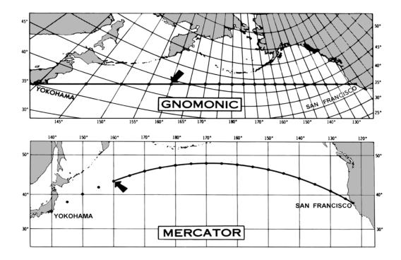
Figure 2404. Constructing a great circle track on a Mercator projection.
