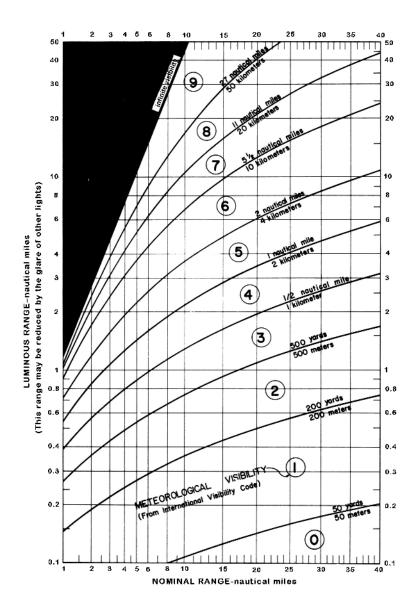
Figure 407a. Luminous Range Diagram.
