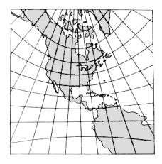
Figure 316b. An oblique gnomonic map with point of tangency at latitude 30°N, longitude 90°W. that any great circle appears on the map as a straight line, giving charts made on this projection the common name **great-circle charts**.
