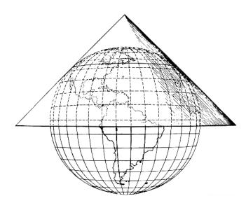
Figure 312a. A simple conic projection.
