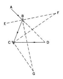
Figure 1601. Optical principle of the marine sextant.
