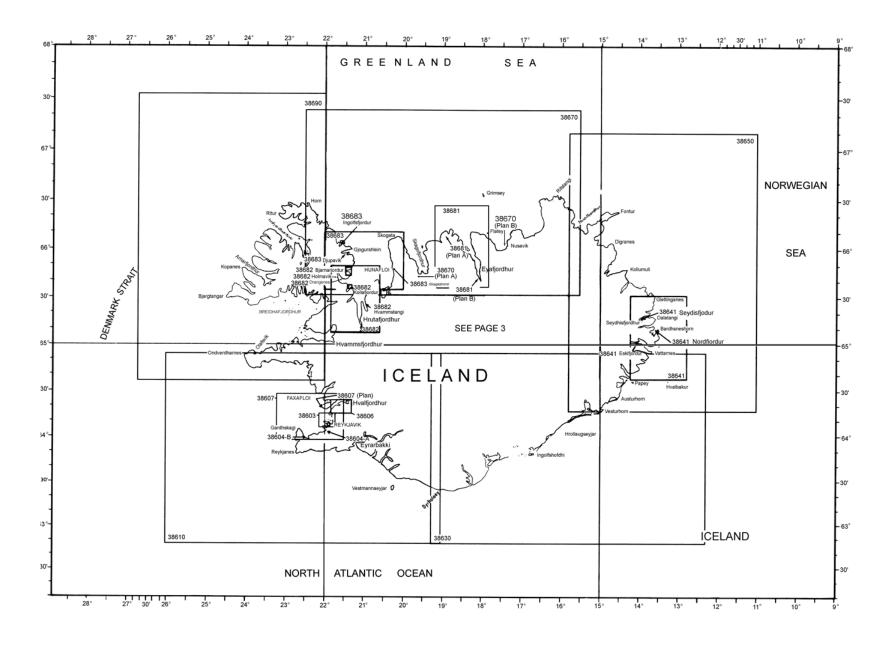
Figure 343c. Chart coverage of Iceland, illustrating the sequence and direction of the U.S. chart numbering system.
