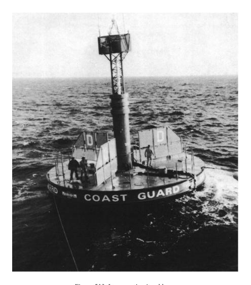
Figure 513. Large navigational buoy.
