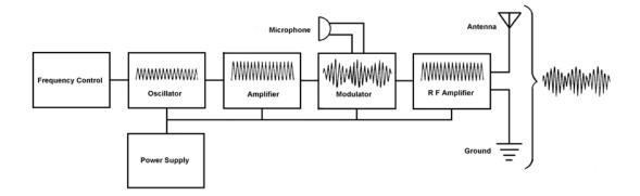
Figure 1016. Components of a radio transmitter.
