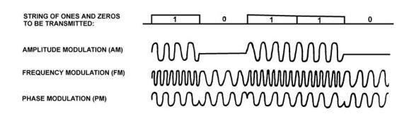
Figure 1104a. Digital data transmission with amplitude, frequency and phase modulation.
