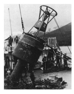
Figure 509. Buoy showing counterweight.
