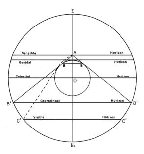
Figure 1526. The horizons used in navigation.
