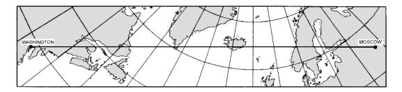
Figure 309d. An oblique Mercator map based upon a cylinder tangent along the great circle through Washington and Moscow. The map includes an area 500 miles on each side of the great circle. The limits of this map are indicated on the Mercator map of Figure 309c.
