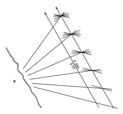
Figure 819b. A number of running fixes with a following current.
