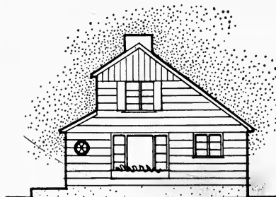
EAVE LINE LOWERED OVER ADDITION
