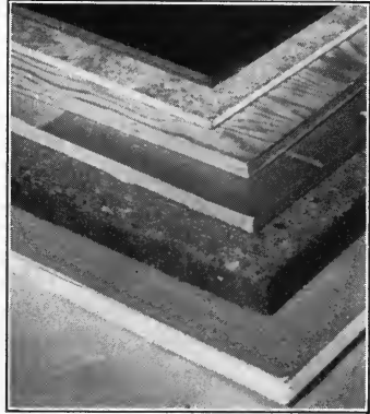
Figure 143. Types of building sheets used in house construction: From top to bottom: hard panel, cement-asbestos, plywood, pressed fiberboard, rigid insulation board, gypsum board.
