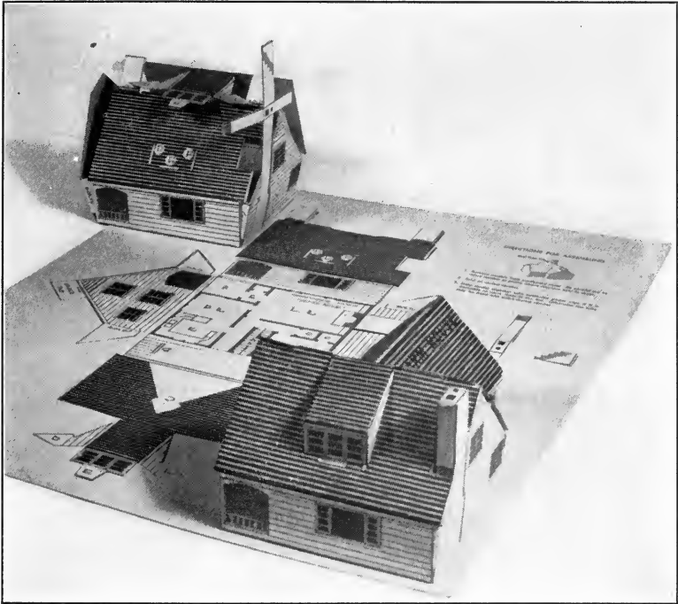
Figure 19. Folded 3-dimension model of a house. Center : flat sheet, cut and creased; rear : partly folded; front : the finished model.
