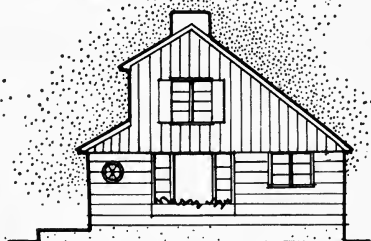
WALL MATERIAL CHANGED ABOVE WINDOW HEAD
