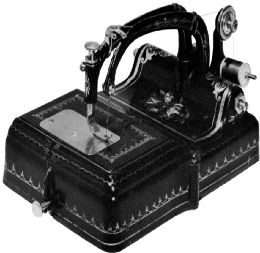
Figure 106.—Lathrop sewing machine of about 1873. These machines were manufactured by the Lathrop Combination Sewing Machine Co. under the patents of Lebbeus W. Lathrop of 1869, 1870, and 1873. The machine used two threads, both taken from spools; moreover, it produced not only the double chainstitch, but it was constructed to produce also a lockstitch and a
