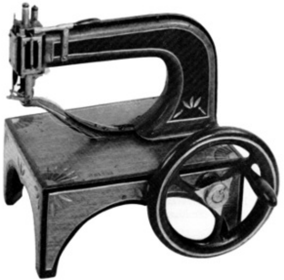
Figure 55.—Blake's leather-stitching machine patent 1858; the inventor claimed the arrangement of the mechanism to be an auxiliary arm capable of entering the shoe, which enabled the sole to be stitched both to the inner sole and to the upper of the shoe. (Smithsonian photo 50361.)
