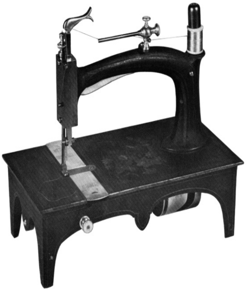
Figure 109.—Lester sewing machine of about 1858. The Lester machine was first manufactured by J. H. Lester in Brooklyn, New York. His machine was based on the patents of William Johnson, John Bradshaw and others but not on the patents held by the “Combination,” although he
