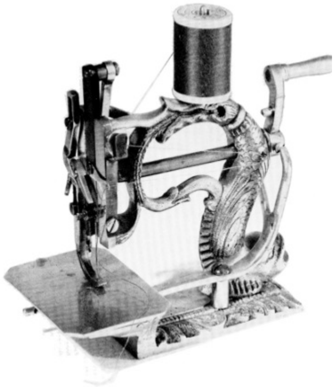
Figure 40.—A dolphin sewing machine based on Clark's This design was first used by T. J. W. Robertson in patent issued on May 22 of that year no claim wa machine design, only for the chainstitch mechanism. The used by D. W. Clark in several of his chainstitch pate made no claim for the design, stating that the machine ‘ any desired ornamental form.’ The dolphin-style n chainstitch models of solid brass, originally gilt. Altho five inches long, they are full-size machines using a
