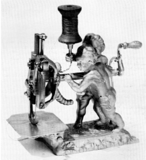
Figure 41.—The cherub sewing machine was another Robertson first which was adopted by Clark. Robertson's patent of October 20, 1857, once again makes no claim for the design; neither does Clark's patent of January 5, 1858, illustrated here. The machine is approximately the same size as the dolphin and is made in the same manner and of the same materials. Two cherubs form the main
