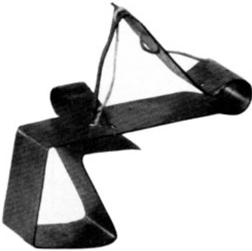
Figure 48.—Heyer's pocket sewing machine patent model, November 17, 1863. This patent model is one piece, and measures about two inches in height and two inches in length. It will stitch—but only coarse, loosely woven fabrics. As can be expected, a great deal of manual dexterity is required to compensate for the omission of mechanical parts. Heyer advertised patent rights for sale, but evidence of manufactured machines of this type has yet to be discovered.
