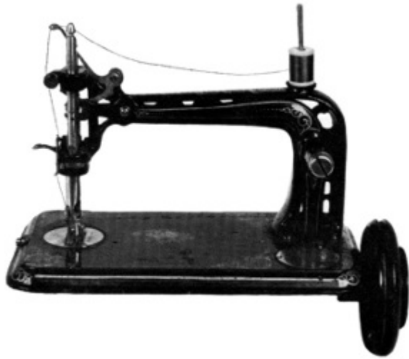
Figure 68. —American Buttonhole, Overseaming & Sewing Machine of about 1870. Using serial numbers, these machines can be dated approximately as follows: 1-7792, 1869; 7793- 22366, 1870;
