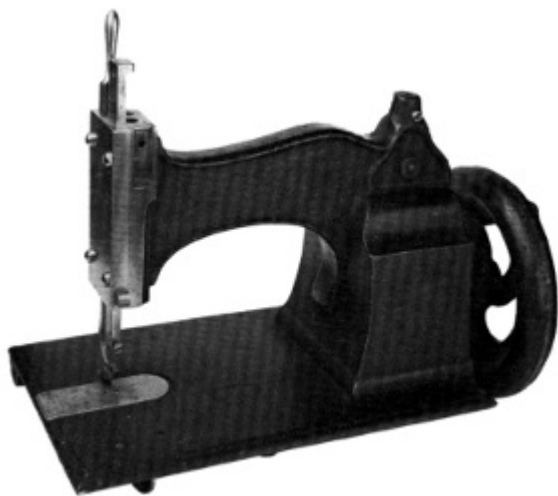
Figure 79. —Clark's Revolving- Looper double- thread sewing machine, 1860. This machine was manufactured by Lamson, Goodnow, & Yale of Windsor, Vermont. It was an attempt to improve on the
