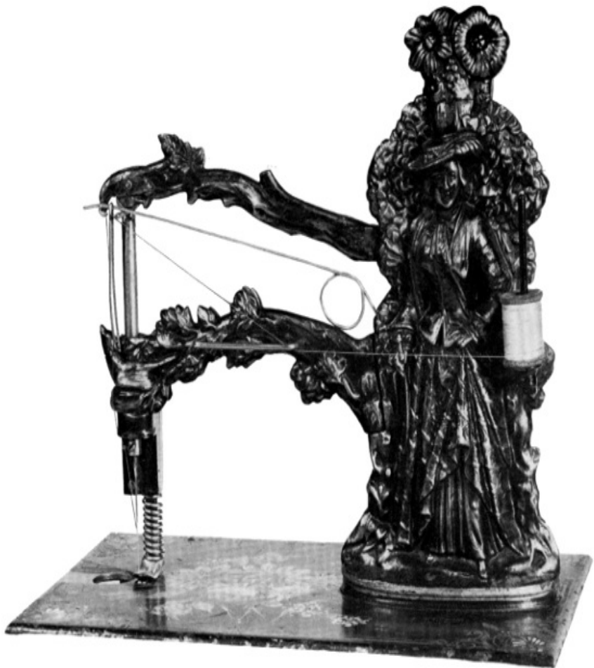
Figure 104.—“Lady” sewing machine of about 1859. The contemporary name of this machine is unknown. The unusual design of the head, or main support, is based in part on the design patent, number 216, of Isaac F. Baker, issued April 10, 1849, for a “new and useful design[,] for
