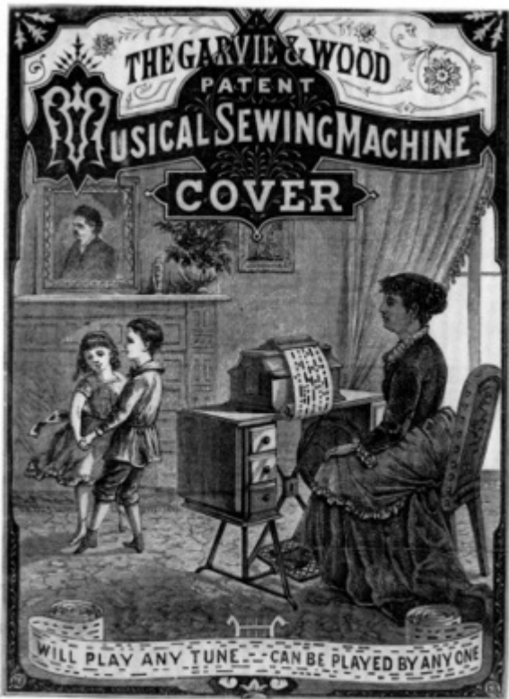
Figure 64. —The treadle of the machine was also used to play music. George D. Garvie and George Wood received a patent on Nov. 21, 1882, for “a cover for a sewing machine ]
