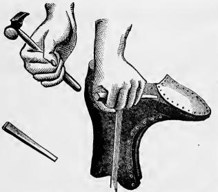
Retailers not accustomed to mending Standard Screw Fastened Boots try to rip off the partly worn sole as they do in mending rivetted shoes. To show Retailers how to mend Standard Screw Fastened Shoes as readily and cheaply as rivetted or sewed shoes, we illustrate by the cut how to take off the partly worn-out sole.
