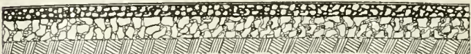
After Covering Material Has Been Spread Over Seal Coat and Then Rolled.
