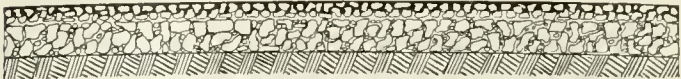
Large Stone for Wearing Surface After Application of Asphaltic Cement. Amount of Asphaltic Cement is from 1¾ to 2¼ Gals. per Sq. Yd.
