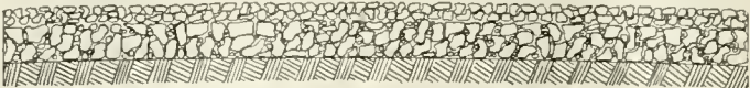
Large Stone for Wearing Surface Spread and Rolled Over Foundation. The Size of This Stone is From 1 to 2½ ins., and is Consolidated to a Minimum Depth of 2½ ins.
