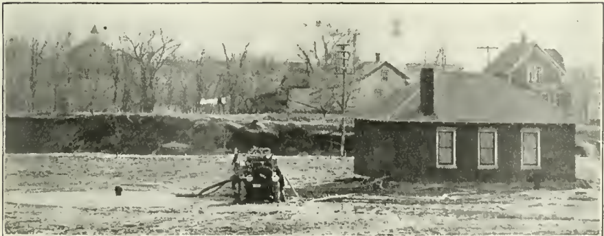
PUMPING WATER SUPPLY OF CLINTONVILLE, WIS., DURING EMERGENCY WITH F W D FIRE TRUCK.
