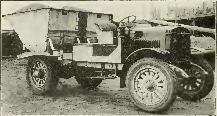
THE KISSEL DUAL HOPPER ROAD BUILDER WITH LEE BODIES.
