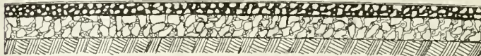
After Application of Seal Coat of Asphaltic Cement. Amount of Asphaltic Cement Applied is from ¼ to ½ Gal. per Sq. Yd.
