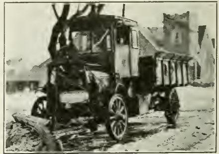
CHAMPION SNOW PLOW ATTACHED TO A G M C TRUCK CLEARING SNOW FROM BROAD STREET, KENNETT SQUARE, PA.
