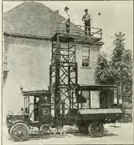
"STANDARD" 2½-TON HYDRAULIC ELEVATED TROLLEY TOWER TRUCK.
