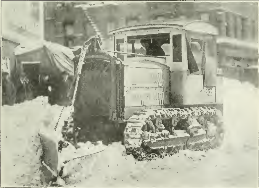
CHAMPION SNOW PLOW ATTACHED TO A HOLT TRACTOR CLEARING SNOW FROM STREETS OF NEW YORK CITY.
