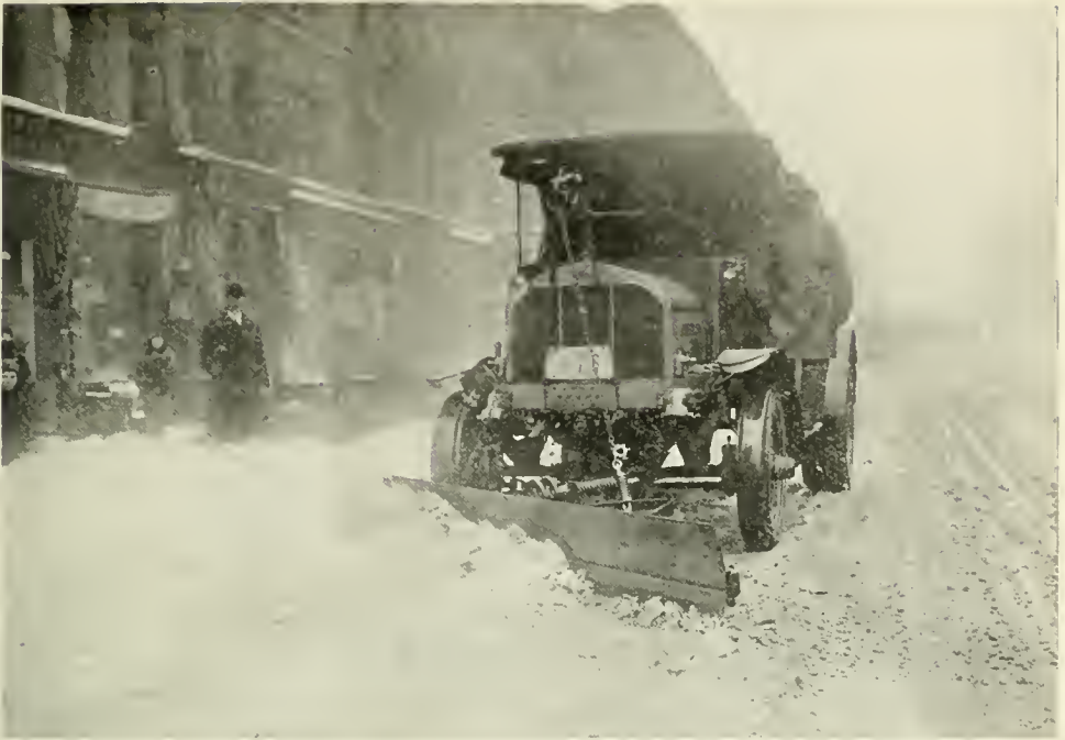
Champion Snow Plow attached to a Sauer Truck. Used by the City of Brooklyn, N. Y.
