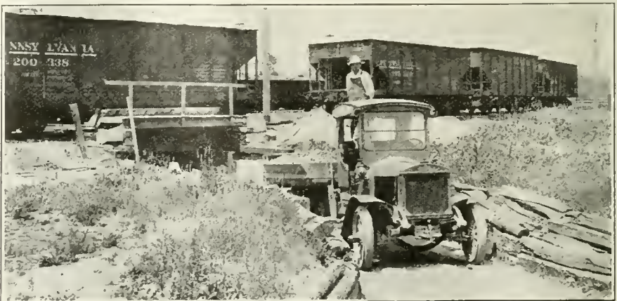
ONE IN A FLEET OF THREE ACME 3½-TON TRUCKS AS OPERATED BY ALLEN COUNTY, IND., ON ROAD WORK.
