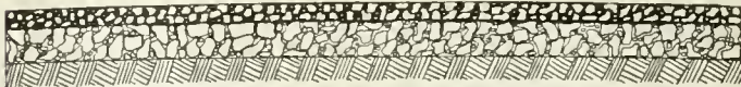
Wearing Surface After ¾-in. Stone Has Been Spread and Consolidated by Rolling.
