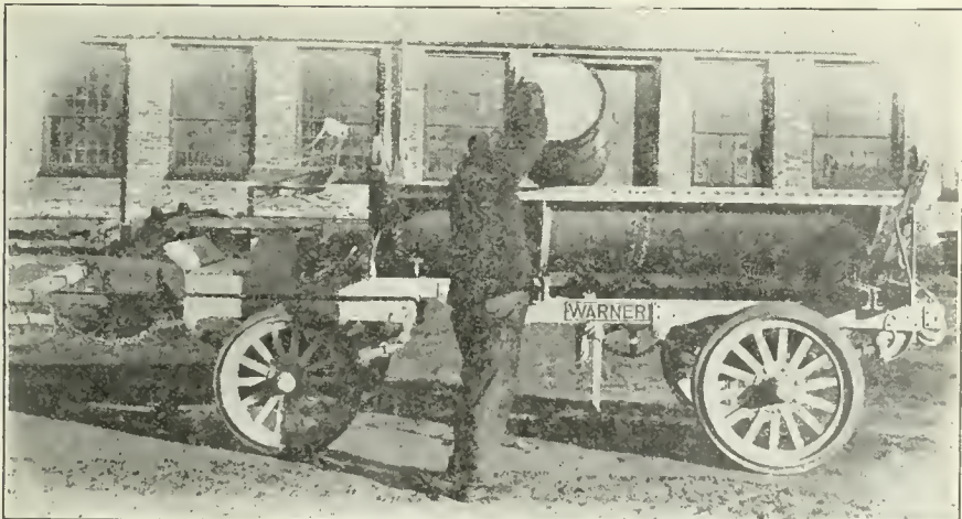
NEW TWO-WAY SIDE DUMP BODY FOR HAULING ASHES AND GARBAGE.
