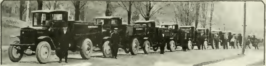
Fleet of 10 Special Kessel Road-builders' Trucks - capacity 3 batches of one yard each.
