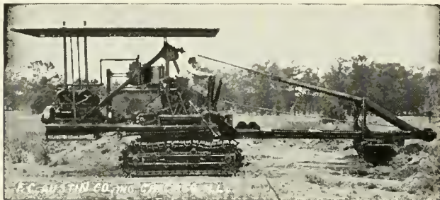
AUSTIN COMBINATION DRAGLINE WITH COMBINATION BOOM AND "SKIMMER."
