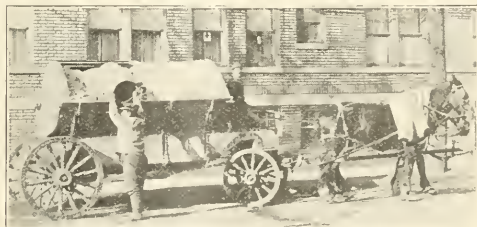
NEW SANITARY METAL ASH WAGON COVER WITH FOUR SEPARATE SLIDING COVERS, USED BY CITY OF NEWARK, NEW JERSEY.
