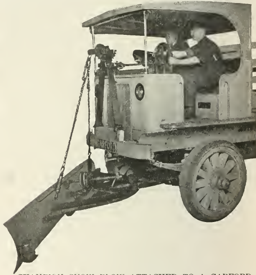
CHAMPION SNOW PLOW ATTACHED TO A GARFORD MOTOR TRUCK.
