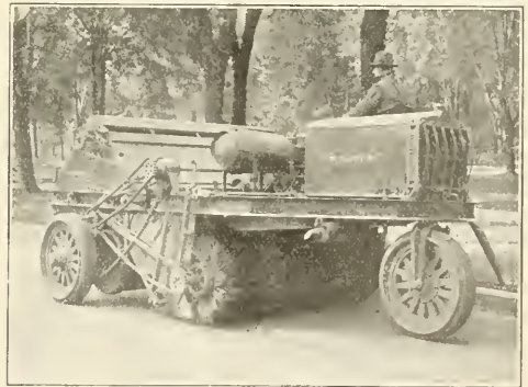
ELGIN MOTOR STREET SWEEPER IN OPERATION ON S. CAPITAL AVE., LANSING, MICH.
