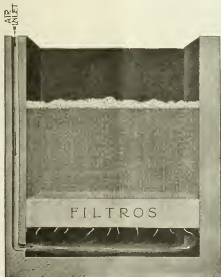
DIAGRAM SHOWING OPERATION OF FILTROS AIR DIFFUSING PLATE.
