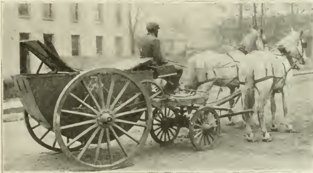
VIEW OF HOLZBOG SANITARY WAGON, USED FOR HAULING WET GARBAGE, ETC. CIRCULAR TYPE OF BOTTOM FACILITATES CLEANING.
