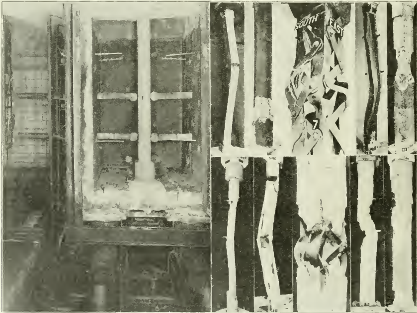
TESTING FURNACE AND ACCESSORIES WITH COLUMN READY FOR FIRE TEST. EFFECT OF LOAD AND FIRE ON SOME SAMPLE COLUMNS TESTED.
