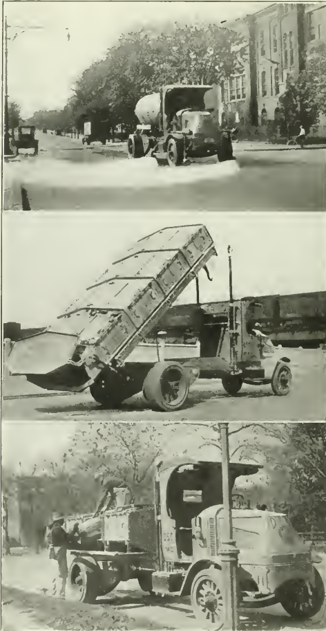
COMBINATION FLUSHING-SPRINKLING-REFUSE COLLECTION MOTOR TRUCK OF TYPE OPERATED BY NEW YORK DEPARTMENT OF STREET CLEANING.
