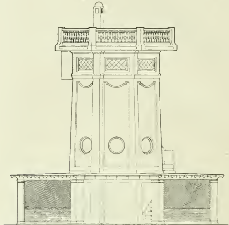
ARCHITECT'S DRAWING OF EASTWOOD REINFORCED CONCRETE OBSERVATORY AND WATER TANK—TOWER AT MIAMI, FLA.
