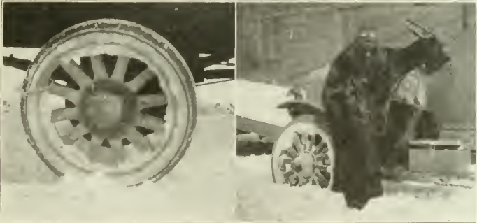
EQUIPMENT HINTS FOR LONG DISTANCE TRUCKING IN WINTER. LEFT: A FAIR EXAMPLE OF HOW WHEELS ARE, BUT SHOULD NOT BE, EQUIPPED WITH CHAINS. RIGHT: A MOTOR TRUCK DRIVER DRESSED FOR A LONG, COLD DRIVE.
