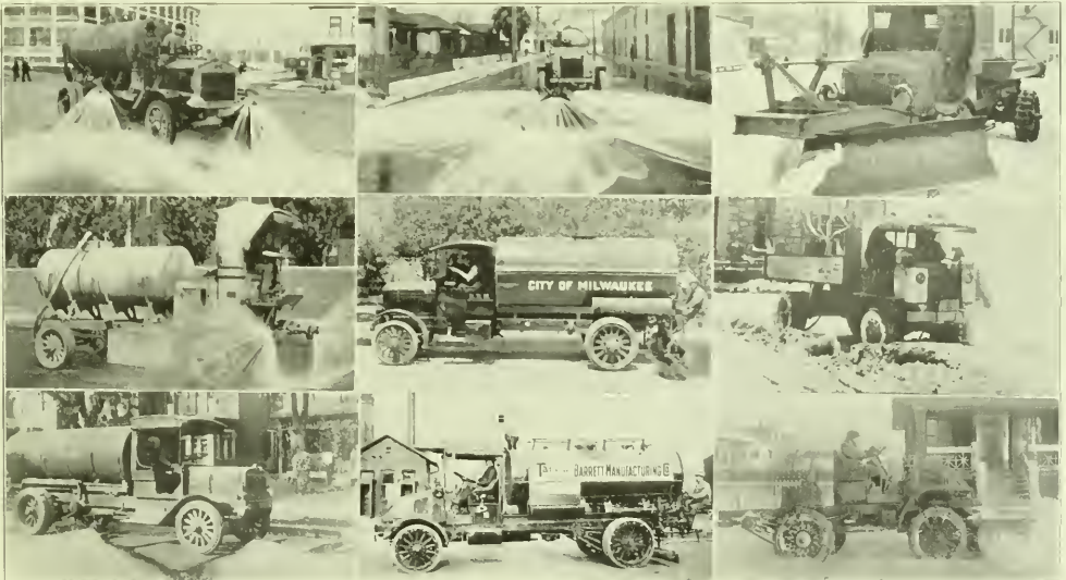
G M C 5-TON FLUSHER AS OPERATED BY THE BARRETT CO., FALLS, N. Y.
