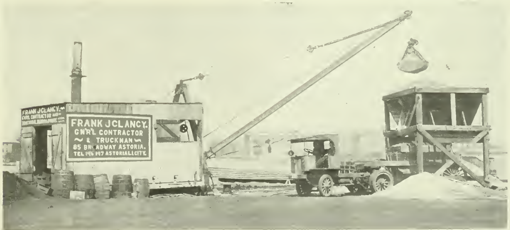
GARFORD TRACTOR (SAME AS ABOVE) PULLING SEMI-TRAILER LOADED WITH SAND (OR GRAVEL). MR. CLANCY STATES THAT THIS TRACTOR EASILY DOES THE WORK OF SEVEN HORSES. IT IS ALSO A "MOTOR MULE," AS SHOWN IN ILLUSTRATION AT TOP OF THIS PAGE.
