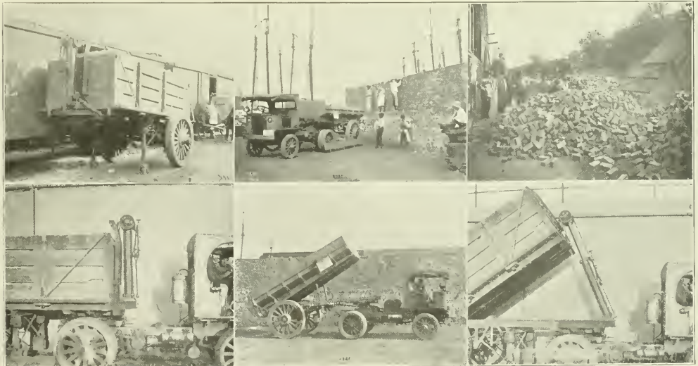
GARFORD TRACTOR AND SPECIALLY DESIGNED TRAILER AS OPERATED BY THE STANDARD BUILDING SUPPLY CO., BROOKLYN, N. Y., IN TRANSPORTATION AND UNLOADING OF BRICK.
