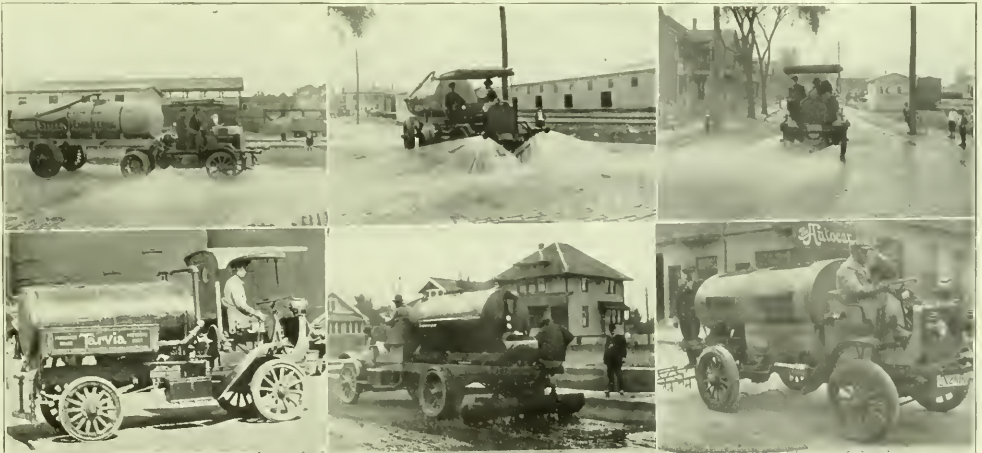
KNOX MODEL NO. 35 FOUR-WHEEL TRACTOR (PULLING HVASS STREET FLUSHING TRAILER) AS OPERATED BY THE CITY OF SPRINGFIELD, MASS. AUTOCAR TAR DISTRIBUTOR AS OPERATED BY THE BARRETT CO., PHILADELPHIA, PA. KELLY ROAD OILER AS OPERATED BY DEPARTMENT OF PARKS, CITY OF OMAHA, NEB. AUTO-CAR OILER AS OPERATED BY DANIELS ROAD OILING CO., PROVIDENCE, R. I.
