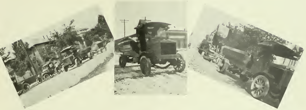
FEDERAL 3 1/2-TON DUMP TRUCK AS OPERATED BY ALDENBROOK, CONTRACTOR, NORFOLK, VA., IN HAULAGE OF OVER 3,000,000 POUNDS PER MONTH AT A COST PER TON OF 15 CENTS.
