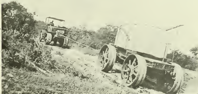
KNOX TRACTOR, AS OPERATED BY THE VERMONT MARBLE CO., SAN SABA, TEXAS. THIS VIEW SHOWS WINCH POWER OF TRACTOR BEING USED TO PULL 12-TON BLOCK OVER A STEEP PITCH ON A POOR ROAD.
