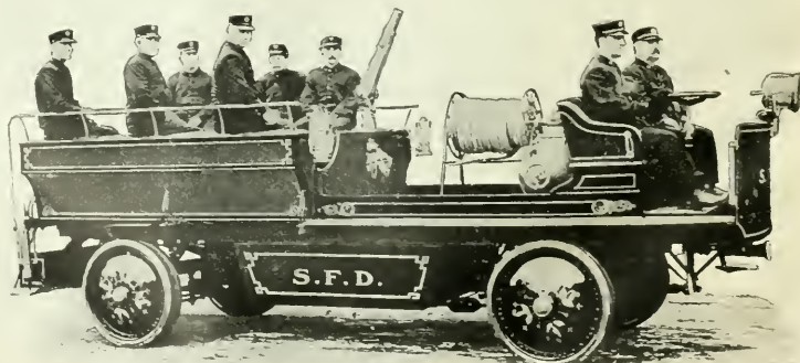
COUPLE-GEAR 3½ TON HOSE AND CHEMICAL (BATTERY-DRIVEN), AS OPERATED BY THE CITY OF SPRINGFIELD, MASS.
