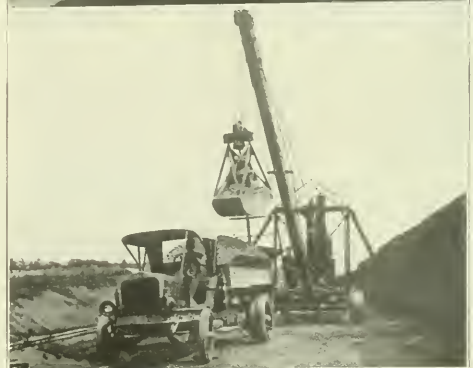
BYERS AUTO-CRANE LOADING TRUCKS ON CHICAGO TEAM TRACKS. TRUCKS AT WORK ARE THE TRUCKS THAT PAY. A TRUCK CANNOT WAIT LIKE A TEAM WITHOUT EXCESSIVE COST FOR LOADING AND UNLOADING. QUICK LOADING AND UNLOADING ARE THEREFORE ESSENTIAL REQUISITES TO THE ECONOMICAL OPERATION OF MOTOR TRUCKS. ECONOMICAL TRUCK OPERATION REQUIRES HAULING CONDITIONS WHICH MAKE THE RATIO OF RUNNING TO STANDING TIME LARGE.
