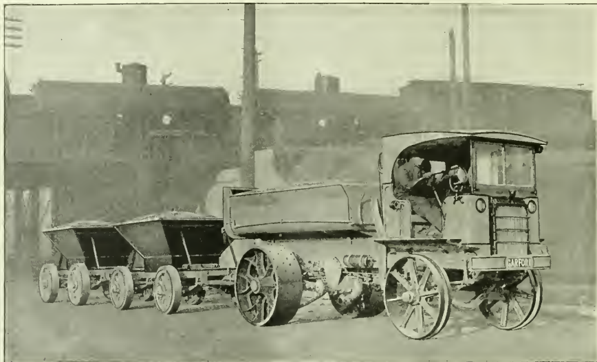
Six tons on truck—five tons on each trailer—total 16 tons
