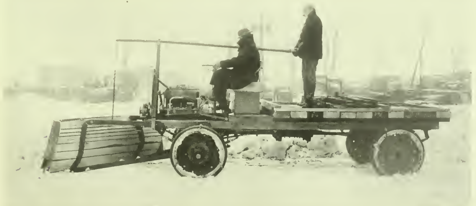
A JEFFERY QUAD WITH A "SNOW SCOOT" CLEARING AWAY A WEEK-OLD SNOW.
