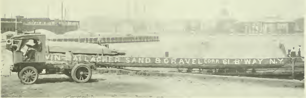
GARFORD TRACTOR, AS OPERATED BY FRANK J. CLANCY (CONTRACTOR), ASTORIA, LONG ISLAND CITY, N. Y. THIS VIEW SHOWS TRACTOR TOWING LOADED SCOWS TO DESIRED LOCATION FOR UNLOADING, THUS SAVING TUG HIRE AND DEMURRAGE CHARGES AMOUNTING TO $90 PER DAY.
