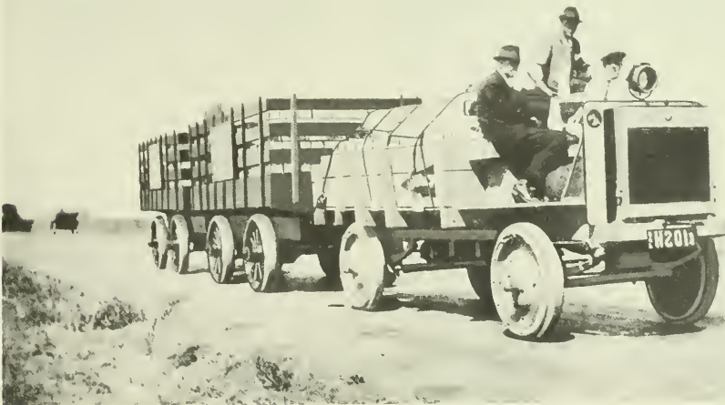
JEFFERY QUAD HAULING 22,410 POUNDS FOR THE MOTOR TRUCK AND TERMINAL COMPANY FROM LOS ANGELES TO SAN PEDRO HARBOR, CAL.
