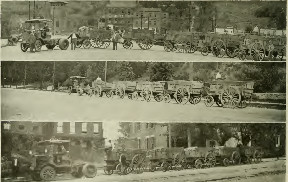
VIEWS SHOWING KNOX TRACTOR. (1) Making complete turn with five loaded trailers; (2) making 6\frac{1}{2} per cent. grade with 38,550-pound load; (3) descending 7.8 per cent. grade at 3 miles per hour, tractor brakes holding back entire 38,550-pound load.
