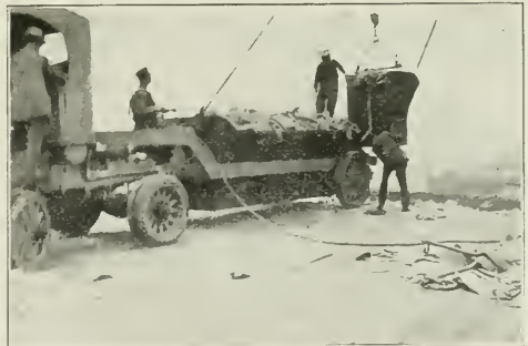
LIFTING WATER-TIGHT CANS of refuse from garbage collection truck to discharge into scow. Gas-electric tractor at the left.
