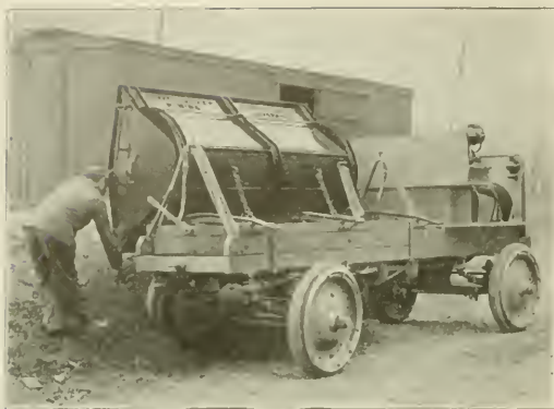
LEE DUMP BODY, Showing Three Rails on Which Body Rolls When Dumping.
