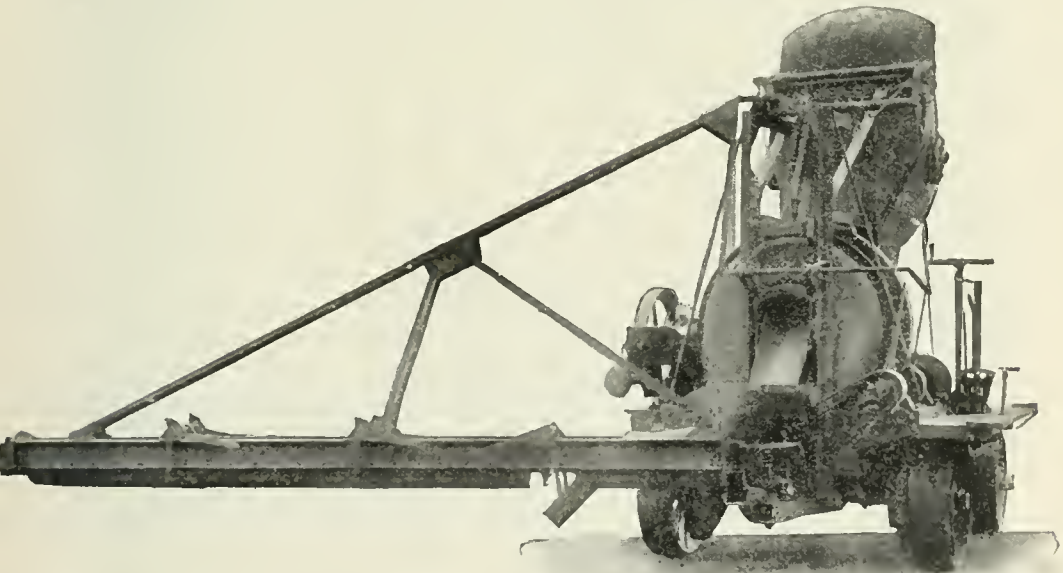
M —C PAVING MIXER, showing distributing trough, discharging at four points along its length.
