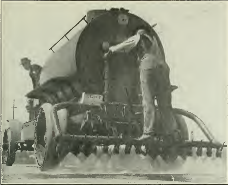
PASADENA TRUCK spraying water on test run, showing shape and overlap of jets, and features of mechanism.
