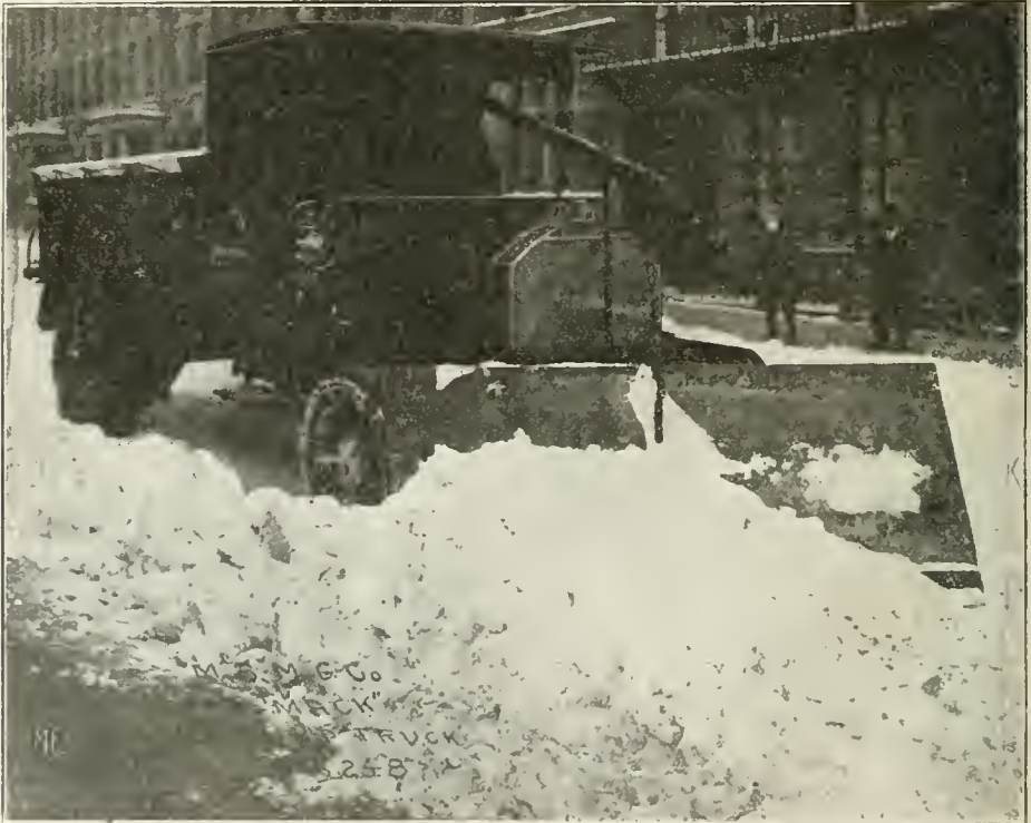
MOTOR TRUCK AS SNOW PLOW, did the work of two hundred men.
