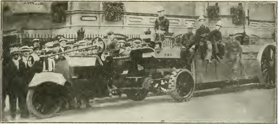
LOW BED GARBAGE TRUCK hauled to dump by Knox-Martin tractor. Horses haul the rear bed from house to house for collection of garbage which when full is exchanged for an empty one brought by the tractor. Exchange easily made by jacking up front end of bed.
