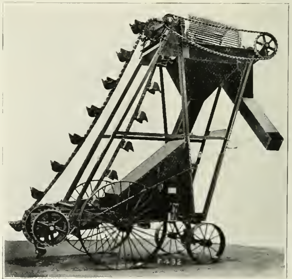
3. EQUIPPED with rotary screen and especially adaptable for repaving work.
