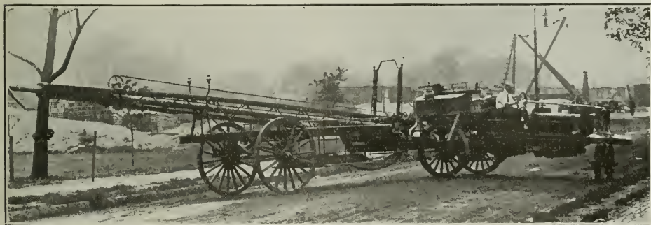
THE MARTIN TRACTOR TURNING AROUND IN A THIRTY FOOT STREET WITH ROOM TO SPARE.
