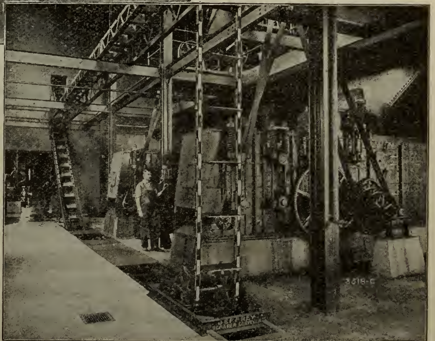
VI. FIRST FLOOR. SHOWING PRESSES DELIVERING DRY GARBAGE TO THE SCRAPER CONVEYOR.
