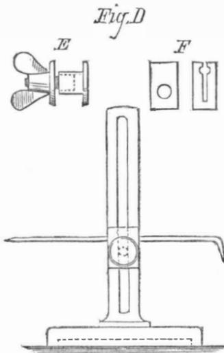
the block complete, the scribe being a simple piece of round steel wire. The dotted line on the foot is the distance to which the foot is hollowed out to make it stand firm. Fig. E is the bolt and nut; the bolt has a flat side filed on each side of it to fit it to the slot in the scribing block stem, so that the bolt cannot turn when it is being tightened. Fig. F is a face and edge view of the piece or clamp for the scribe which passes through the hole in the slot.
