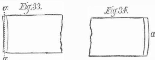
them by the cut, which, acting as a wedge, endeavors at each blow to drive them outwards instead of inwards, as would be the case in a properly shaped chisel, as shown in Fig. 34, *a* being the cutting edge.
