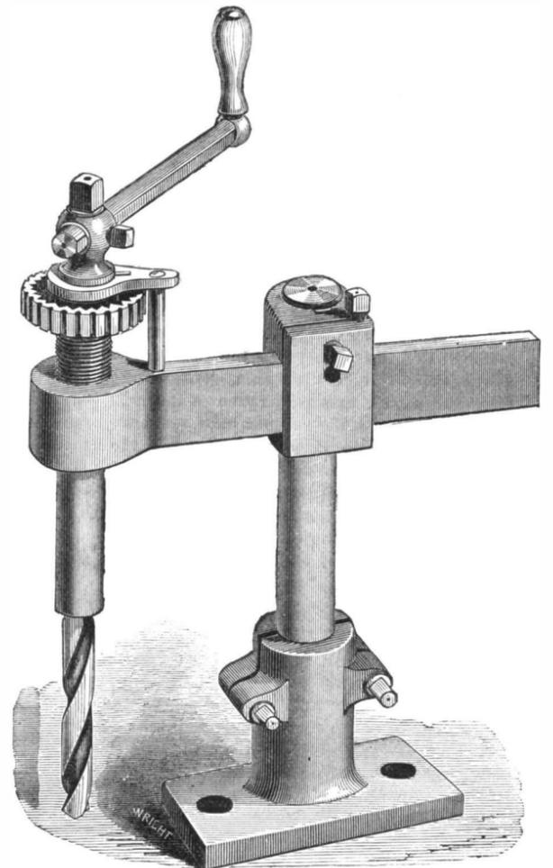
A change of spindle can be made almost instantly to suit drills of different shanks, and if desired a hand feed can be used. The arrangement for holding the standards is such that, with any reasonable degree of care, it will not be marred.
