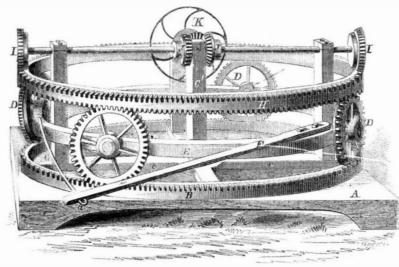
to the central upright, C'. The bevel wheels. S, give motion through another one to the belt wheel, K, by which the power can be conveyed to any machine desired. By varying the proportions of these wheels, any desired relation between the velocity of the horse and | Park-place, New York.
