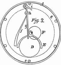
having a cylidrical weight placed within its case, said weight being detached, and from its gravity remaining stationary (not revolving with the wheel) and thereby giving motion to the working parts, as the wheel re-
