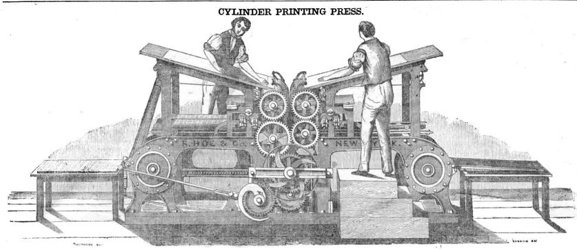
The above engraving represents one of R. Hoe & Co.'s double cylinder printing presses. They are capable of throwing off from four to five thousand impressions per hour. The types are placed on a solid, cast iron plate, or bed, the motion of which is horizontal and reciprocating. The sheets of paper being put in the proper position, are caught by means of small cast iron fingers which are attached to and revolve with the cylinder, and are thus
