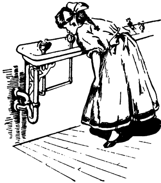
Figure 66. — Sanitary fountain in one of the Houston schools.
