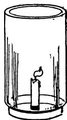
Figure 118.—A candle will go out for lack of oxygen if covered with a jar.
