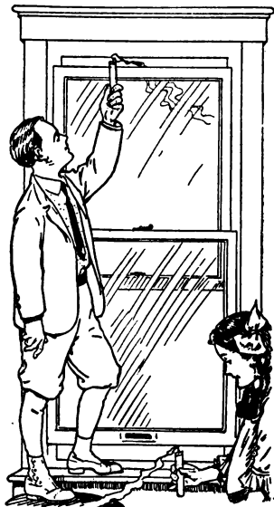
Figure 135. — Experiment to show outgoing current of warm air and incoming current of cold air at a window.
