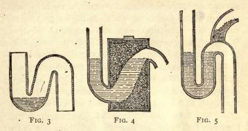
partially exhausts the air in all the branch pipes. The pressure of the atmosphere outside the pipe, upon the water in the trap, will then be greater than that from inside the pipe, and the water in the trap will be forced down into the pipe, until the water seal is broken and space left for the passage of foul air up into the room.
