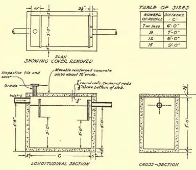
FIG. 24.—SUGGESTED DESIGN FOR A SINGLE-CHAMBER SEPTIC TANK
