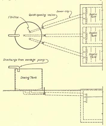
FIG. 5.—PLAN AND ELEVATION OF THE DOSING APPARATUS This dosing tank was used to divide the flow of sewage into the one-, two-, and three-chamber tanks (A, B, and C) shown in Fig. 4.
