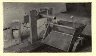
Fig. 1.—Tipping-Bucket Meter for Determining the Quantity and Rate of Sewage Flow From a Farm Home
