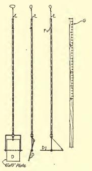
FIG. 8.—DEVICE FOR MEASURING THE THICKNESS OF SCUM
