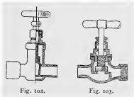
there would be a square end over which a loose key would fit. Stop valves should be provided both outside and inside the building.
