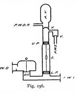
A diagrammatic section of a ram on the double-acting
