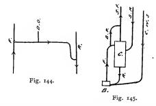
from the one to the other as shown in Fig. 144. In such a case, the slight fall generally available for the pipe is insufficient to ensure a good circulation through this extra pipe, and matters are put right by giving the pipe a "drop" as shown, the greater density of the water at the lower part of the drop increasing the velocity of flow through the pipe. D.O. = draw off.
