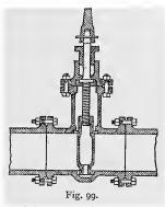
raises or lowers the sluice by means of the screw shown.
