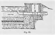
stone slab to prevent the disturbance of the sand around it. Below the gravel a drain grate of bricks is shown. the floor falling to a sunk main drain in the middle. Such a drain might lead to a small chamber at one end, containing means of re-
