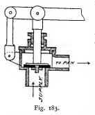
most usual. Some forms of inlet valve do not require regulators, but they are usually complicated in construction and liable to get out of order. Fig. 183 shows the construction of the usual form of water inlet for a valve closet. It will be seen that it is opened by the raising of the lever and closed as the lever goes down again. If a valve closet is to be flushed by means of a waterwaste preventing cistern, the pull of
