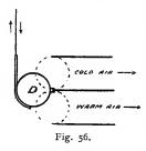
diagrammatically by Fig. 56, which is an outline section through the heads of two subsidiary ducts. The damper D is in the form of a metal cylinder, loosely hinged to the division between the ducts. It can be raised or lowered till it occupies either of the positions shown by the two dotted circles. Thus, when in the position of the upper circle, the cold air is entirely
