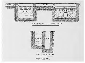
tributing chamber, D.C., a very shallow chamber as shown in Fig. 359.
