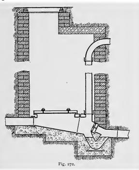
the drain. It will be seen that an air inlet socket is provided at A, and an access stopper at S. This type has been used by H.M. Office of Works on the drains of public buildings near the Thames at Westminster.
