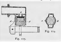
for the water, but this difficulty is overcome by making the section of the casing around the valve in the form shown in Fig. 114. Like the low pressure valve of this type, the high pressure one is noisy, the water entering in two disjointed
