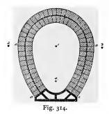
concrete has also been used with success. Fig. 314 shows one method of construction. The invert is formed of terra-cotta blocks which give a minimum of joints at this important point. They are moulded hollow as shown and are usually made with rebated joints. The inner ring of brickwork should be of either salt-glazed or blue Staffordshire bricks, both of which form a
