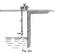
on which is wound a tape measure, at the other. At the end of the tape, T, is a plumb bob, P.B., with a long point. It is allowed to fall slowly till the point touches the water surface and the spindle can then be clamped by a small set-screw, S.S. The apparatus can be lifted up from the side of the manhole and put in its case, no one but the observer knowing the water level.
