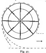
poses, but they are always of metal. It is interesting to note that one of the bestknown types is of very similar construction to that just referred to. Fig. 51 shows a section of what is termed a fan wheel. It is similar in form to a paddle wheel. The thick lines show the blades in section, and they are connected at their sides to flat rims, one of which is shown
