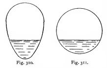
Their respective advantages and disadvantages may be briefly stated. The circular sewer of brickwork is stronger than the egg-shaped, and slightly less expensive to construct, but the egg-shaped
