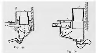
through it, and the flushing effect on the trap is naturally very slight. Fig. 159 shows a different type, in which a tipper,
