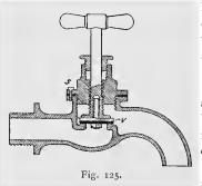
kind. When the tap is closed the passage of the water is prevented by a small valve, V, which consists of a circular disc with a guiding pin above it and a leather washer, shown in black, below it. This valve is kept down by pressure exerted through the screwing down of the handle, the stem of which has a cavity
