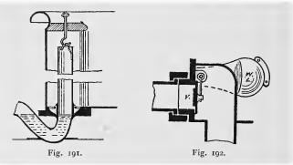
over the mouth of the waste pipe of the lead safe under the bath. The valve leads into a trap, T, which is provided with a ventilating pipe, V.P.
