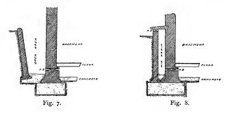
to walk round, paved with concrete rendered in cement and laid with falls to gulleys at intervals. The earth is kept up by a small retaining wall, either sloping as shown in the sketch, or vertical. If the retaining wall is vertical, it requires to be rather thicker near its base. The arrangement of the damp course and air bricks is as already described.
