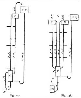
within a larger one, the small one being used as a means of heating the water by contact, and the supply to the fittings not passing through the boiler. Thus there are two complete systems in one. The boiler has the usual main flow and return pipes connecting it to the small cylinder, or indirect heater, which has its own expansion pipe. The water supplied to the fittings is passed through the main cylinder and around the heater, but the temperature does
