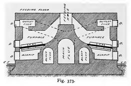
drying hearth has no place in this form. The fire bars are shown by a thick black line as in the previous example. There are three doors to each cell, the top one for cleaning the outlet flue, the next for clinkering, and the lowest for access to the ashpit.
