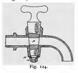
the pipe no water can get through. This form of tap is simple in construction, but closes very rapidly, with the result that it leads to concussion or water hammer in the pipes, the increase in pressure caused thereby having often been sufficient to burst the pipe.
