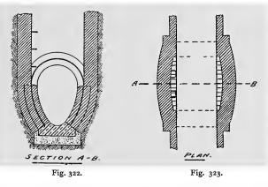
In the case of a larger sewer, the base of the manhole is of different construction. An example of this is shown in Figs. 322 and 323. The latter shows the plan, and the former a cross-section, of a manhole on an egg-shaped sewer. It will be seen that, without making the base of the manhole of exceptional size, there is no appreciable benching, but merely enough to give a foothold. The curved shape of the walls on plan is to give greater strength.
