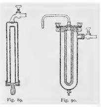
tains the "candle," and is screwed on to the tap. At the bottom is a glazed nozzle outlet. By unscrewing the collar just above this the candle is at once freed for cleansing purposes. Fig. 90 shows the Berkefeld filter, which is of rather different construction. It has a thicker candle formed of baked fossil earth and filters more rapidly, though its
