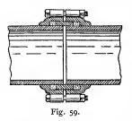
show the general idea. Fig. 59 shows the "Jones" joint, which is formed as follows. The pipes have no sockets, and are butted end to end at a little distance apart to allow for expansion. Around the abutting ends is a flat iron ring, and on either side of this a rubber ring, shown by fine dots in the section. These three rings are
