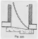
of it would be about at O, and the pipe would pass down to join the outlet sewer a few feet from the manhole. Flap valves sometimes have floats attached to them which are intended to lift them automatically when the sewage reaches a certain height, but the plan is not very reliable.
