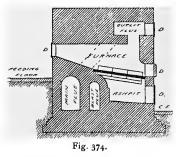
some from the front. An example of a back-fed destructor cell is shown in Fig. 374. It will be seen that this is a modification of the Horsfall type shown in Fig. 373. The furnace is fed from a feeding floor below the top of the destructor. This method is quite sound, as there is no
