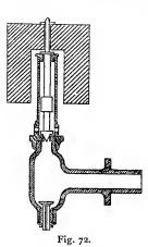
gets beyond the predetermined figure it automatically rises and lets the water out into the tank. On the pressure falling below its normal amount, another small valve, at the bottom of the Fig., automatically rises and lets more water in. The spindle of this valve is not of circular but of cruciform section, so that a very slight rise of the spindle will let water in.
