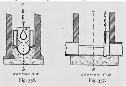
Tipping tanks are also used for flushing sewers, but they are only suitable for small volumes of flow.
