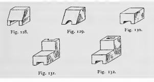
shown in Fig. 132. It will be seen that a maximum of heating surface is obtained in this way. The boot boiler in its ordinary form consists practically of two saddle boilers at right angles, and though more expensive than the ordinary saddle boiler, it will supply about double the quantity of hot water in a given time.
