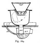
closet shown in Fig. 164. It consists of a conical basin of glazed earthenware, fixed over a large cast-iron container, C, the outlet of the basin, being closed by a hinged copper pan, P, holding water and held up by leverage. The solids fall into the pan, P, and, on pulling up a handle in the seat, the pan falls to the position shown by dotted lines, throwing the con-
