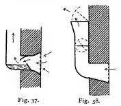
It is constructed with a small bath of water at its base, with baffle plates to deflect the incoming air on to the water surface as shown by the arrowheads. The effect of this is that the particles of dust and grit in the air are caught by the water. The intention is that this shall act as
