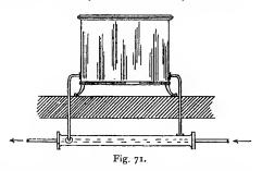
diameter, to the ends of which the ordinary small pipe is connected. From the larger pipe a flow is taken to the radiator, a return being taken from the opposite end. The method of connecting the flow and return has already been described, and should be again noted in Fig. 71, the flow going from the top of the pipe and the return being connected to its side.
