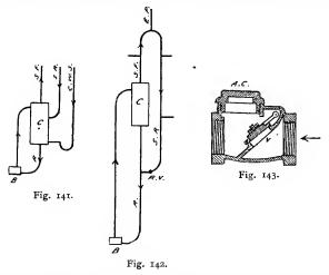
To save making two holes through the chimney breast, the flow and return are often brought through the same hole, both entering the side of the cylinder low down, but in such case the flow pipe must be carried up some distance inside the cylinder.
