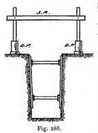
gradient is by the sight rail and boning-rod system. On either side of the proposed drain a drain pipe of good diameter, say 9 inches, is set up as shown at D.P. in Fig. 288. In each of these an upright post is planted, being well packed round with earth or sand. The sight rail, S.R., is then fixed to the two posts. By means of the sight rails an imaginary line is drawn, parallel to the intended gradient of the drain, and this can be easily fixed, no matter whether the gradient be
