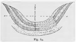
well. Assuming the water level, in the lowermost permeable stratum shown, to be at the line AB, water will rise approximately to that level through the well. The name Artesian is derived from the fact that the first such well was sunk in the province of Artois, in France. One of the earliest Artesian wells in London was that sunk in 1844 to supply the fountains in Trafalgar Square. It goes down 393 feet to reach the upper chalk formation.
