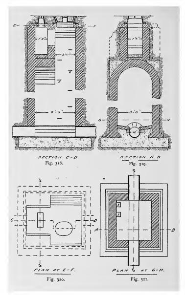
If it is not desired to have a ventilating opening at the level of the street, this part of the detail can be readily omitted.
