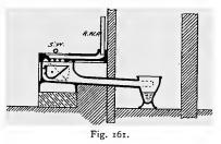
piral flush to the pan. If the tipper happens to discharge when the pan is in use, the user is apt to get splashed, but notwithstanding this, Fig. 161 shows the least objectionable of the four types illustrated. In each case the sketches are diagrammatic, the joints being omitted to simplify the illustration.
