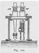
The hole is drilled and tapped, and the cover then revolved to bring the ferrule over the hole, into which it is screwed. A screw-plug is fitted to the ferrule, and this is kept screwed down so as to close the branch, as shown, until the house service is laid on.
