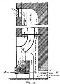
grate, designed for the old War Office, in Pall Mall, by the late Sir Douglas Galton, is an excellent example. Fig. 40 shows a vertical section of this grate. Cold airenters through a grating at the outside face of the wall and circulates in an air-warming chamber behind the fire. It then passes upwards and around the smoke flue, and is admitted into the room by means of two louvred openings at the side of the mantel.
