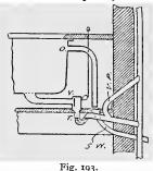
Scullery sinks are best made of glazed fireclay, other materials being unsuitable. They are of two kinds, shallow and deep. The shallow sink has usually a grating outlet and really serves only the purpose of a safe. Having an open grating as outlet it requires no overflow. Scullery sinks are often used as washing-up sinks, and in such case require plug out-
