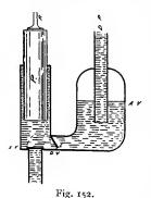
side of Fig. 152. In this form the piston takes the shape of a solid plunger, P, of almost the same sectional area as the barrel. It will be seen that its action is similar to that shown in Fig. 151, the plunger displacing a certain quantity of water each time it descends, and forcing it into the delivery main.
