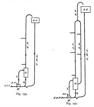
system, provided with a secondary flow and return taken round past the various fittings so as to supply them by means of short branches. Branches are taken from both flow and return pipes of the secondary system of circulation, the secondary flow being marked S.F. and secondary return S.R. The letters already used will be adopted in the remaining
