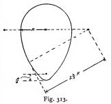
and a half times the greatest horizontal diameter, but the radius of the invert is only half as great (i.e. one-quarter R) as in the
