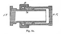
no rubber rings are used; the joint consists of an inner and outer tube (I.T. and O.T.) sliding one within the other. At A is a packing of hemp treated in various
