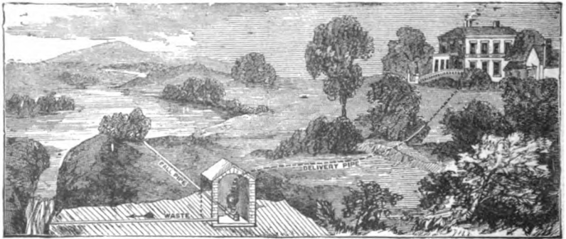
FIG. 356.—Arrangement of hydraulic ram and pipes.
