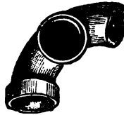
FIG. 26.—Earthenware right-angle bend, with access socket.
