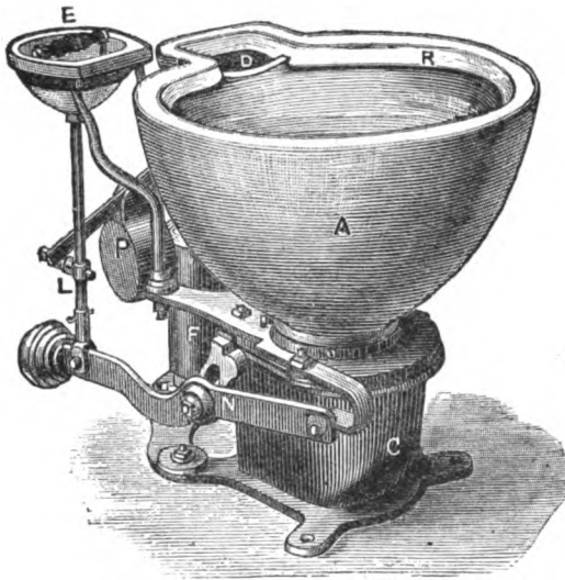
FIG. 186.—Improved valve water-closet.
