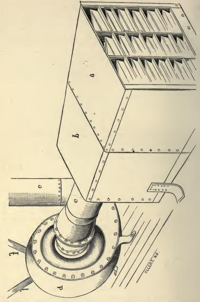
(PLATE 3.) FUMIGATING FURNACE, RESERVOIR, AND EXHAUST FAN.
