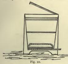
communicates above with the interior of the chamber by a double row of holes around the four sides. The interior of the chamber is connected by a flue at the side by an aperture opening in the centre of the bottom, and capable of being opened and shut from the outside by a sliding valve.
