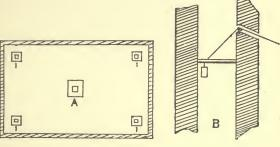
Fig. 17. ed to permit ventila- A .- Plan of roof of chamber. IIII.- Ventilators of isolating spaces. B .-- Section of chimney showing damper.
