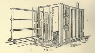
air from the chamber can be made to pass through the furnace. From 60 to 75 pounds of coke are consumed each time of using the apparatus.
