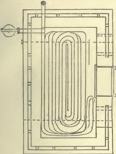
In order to use the apparatus, the articles to be disinfected are hung up on hooks in the chamber. The doors are clos-Fig. 16.—Plan showing arrangement of heating pipes. ed, and the steam turned into the copper steam pipe. The damper in the chimney and the valves of the air tubes are opened for half an hour to allow all moisture to be
