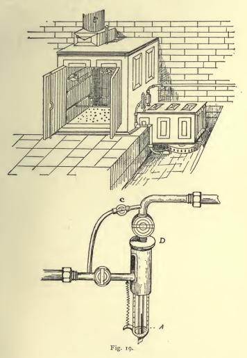
At the top of the chamber there is an outlet flue controlled by a valve, and furnished with a thermometer (E, Fig. 19). In connection with the outlet is an arrangement designed for the extinction of fire. When the temperature at the outlet exceeds 149° C. (300° F.), a link of fusible metal melts, closing a damper, and shutting off the supply of gas. The chamber is fitted with bars and hooks for suspending clothing and other articles to be disinfected.
