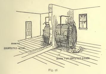
on hinges at one end only, the back being steam jacketed like the circumference. This form was made to run on wheels for removal from place to place, if desired. Another form, designed for a town disinfecting station, and intended to be placed in the partition
