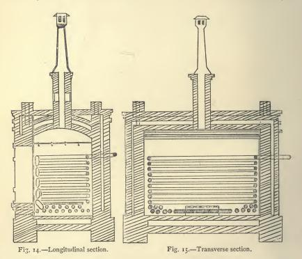
of sawdust is ventilated by ventilators extending above the roof. The interior of the chamber is 7 feet 4 inches high, 9 feet 10 inches long, and
