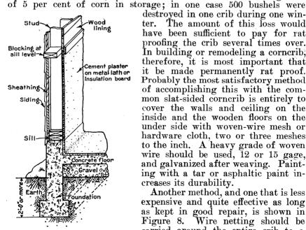
FIGURE 7.-Recommended construc-GURE 7.—Recommended construction of walls and floors of new frame barns. Cement plaster on metal lath or insulating board is applied to the inside of the studs at least to the level of the window sills as a better protection against rats and as being more easily kept clean than wooden lining
