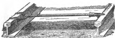
FIG. 305. HUNTINGTON'S TRACK GAUGE. Can also be used to square ties with the rail, though there are roads having a special tool for squaring the ties with the rail.
