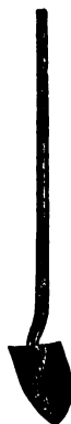
FIG. 303. LONG HANDLED SHOVEL. For digging deep trenches or deep holes as for telegraph poles.
