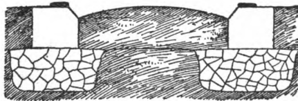
Stone Stringer and Strap Rail, Baltimore & Ohio Railroad, A. D. 1833. This was a favorite American device.
