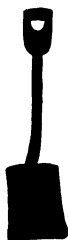
FIG. 301. RAILROAD SHOVEL. For tamping earth, sand and some varieties of gravel ballast and for ditching, etc.
